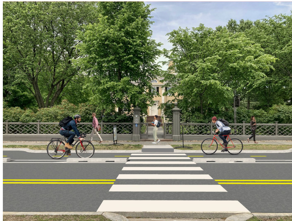
Example image of pre-cast concrete curbs without flex posts
