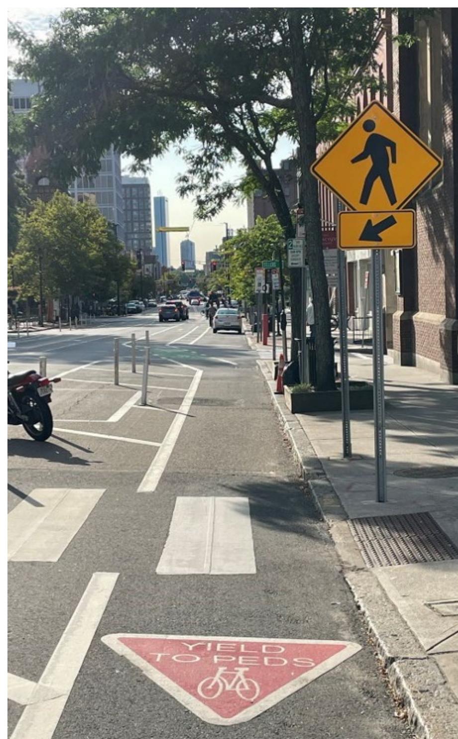
Example: Separated bike lane at crosswalk at Mass Ave at Clinton St
