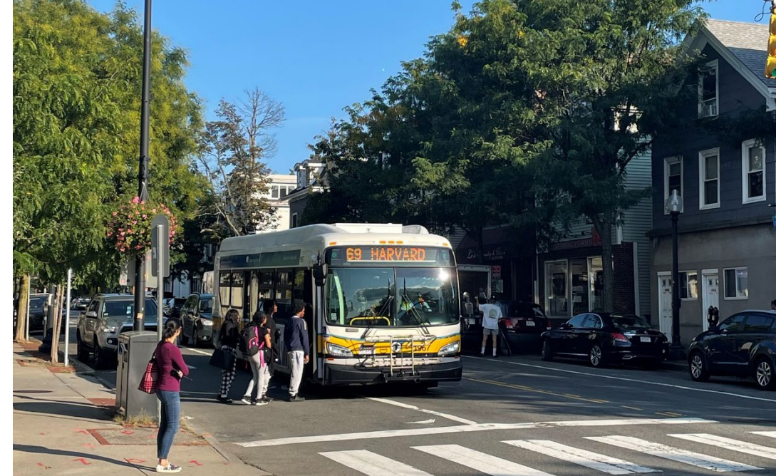
Bus stops that are shorter or before an intersection (as shown) make it harder for the bus to reach the curb. This makes it harder for people to use the accessible boarding ramp, when needed.
