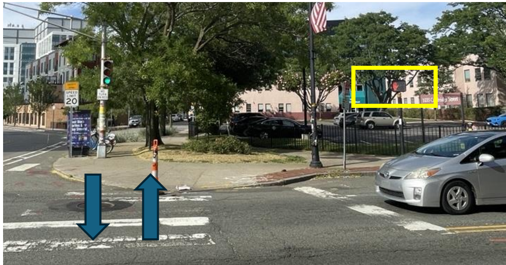
Example of signal equipment that should be relocated. The signal head does not line up with a pedestrian's path of travel.
