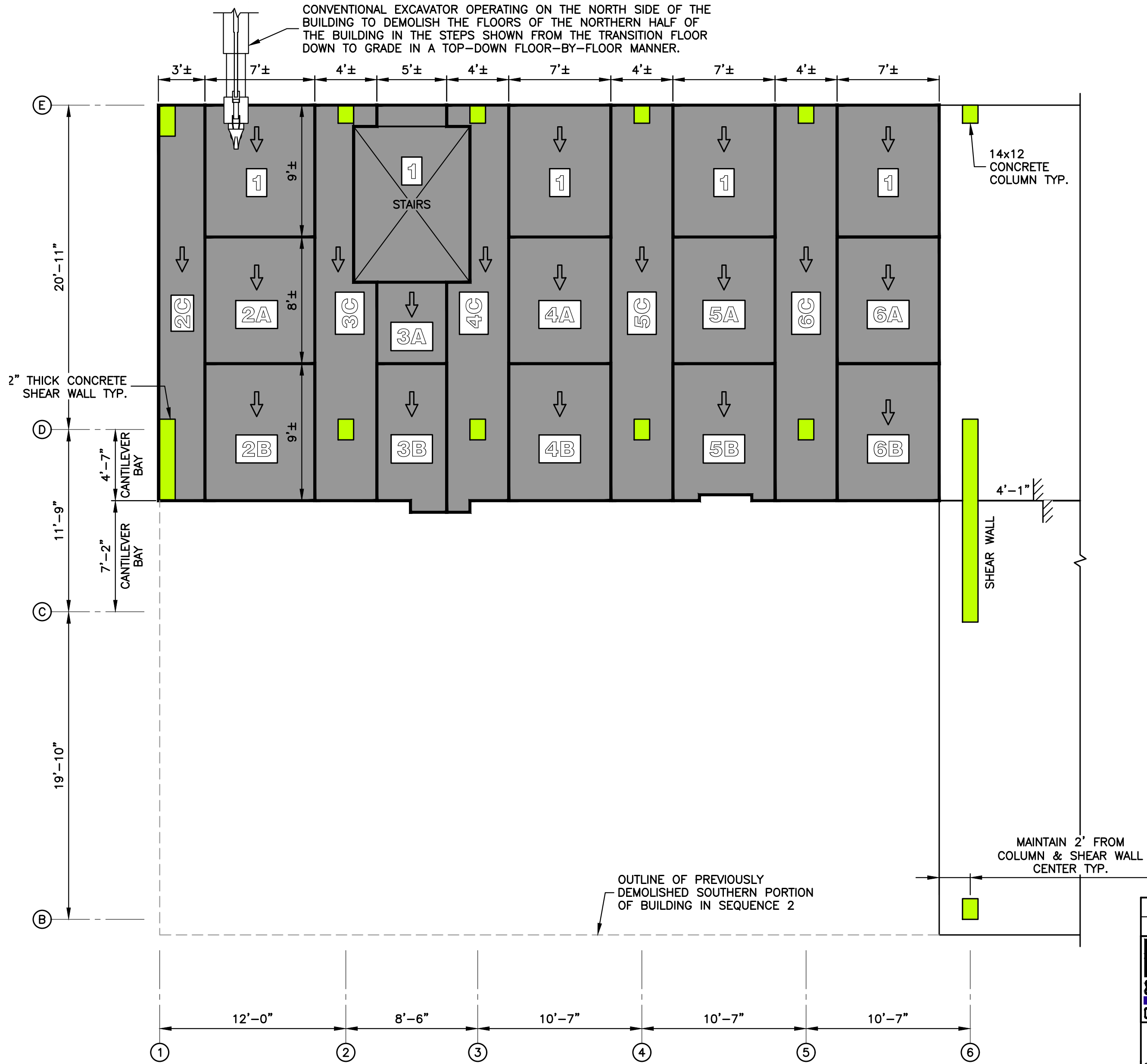
TYPICAL FLOOR DEMOLITION FOR SEQUENCE 4 w/ CONVENTIONAL EXCAVATOR SCALE: 3/16" = 1'-0"
