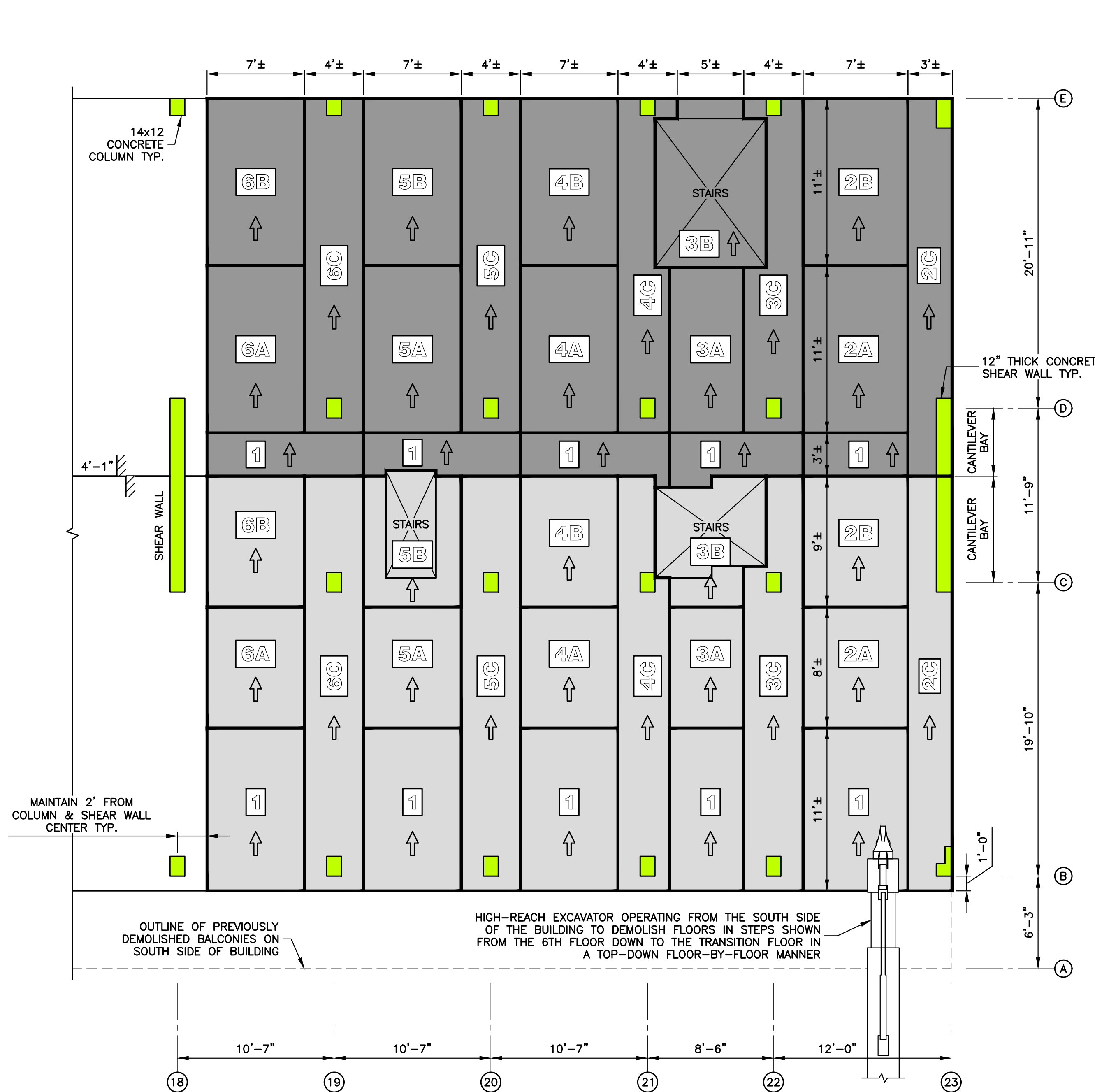
TYPICAL FLOOR DEMOLITION FOR SEQUENCE 3 w/ HIGH REACH EXCAVATOR
