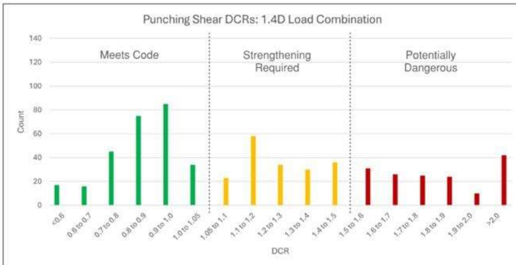
FIG. 2 – Count of slab-column connections by DCR range under dead-load only (structure self-weight), showing categorizations (meets code, strengthening required, potentially dangerous) for the unloaded structure.
