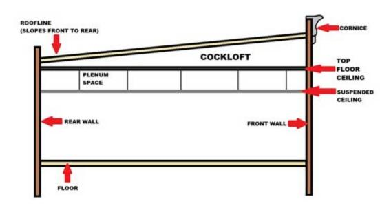
The cockloft is a void space that is created between the top floor ceiling and the roof decking. An inherently common feature in Type III (Ordinary) constructed buildings but can be found in all types of construction. The cockloft is nothing more than a horizontal balloon frame construction. This is an often-unimpeded passageway for fire to travel and spread throughout a building. As discussed in TB 2023-14.
