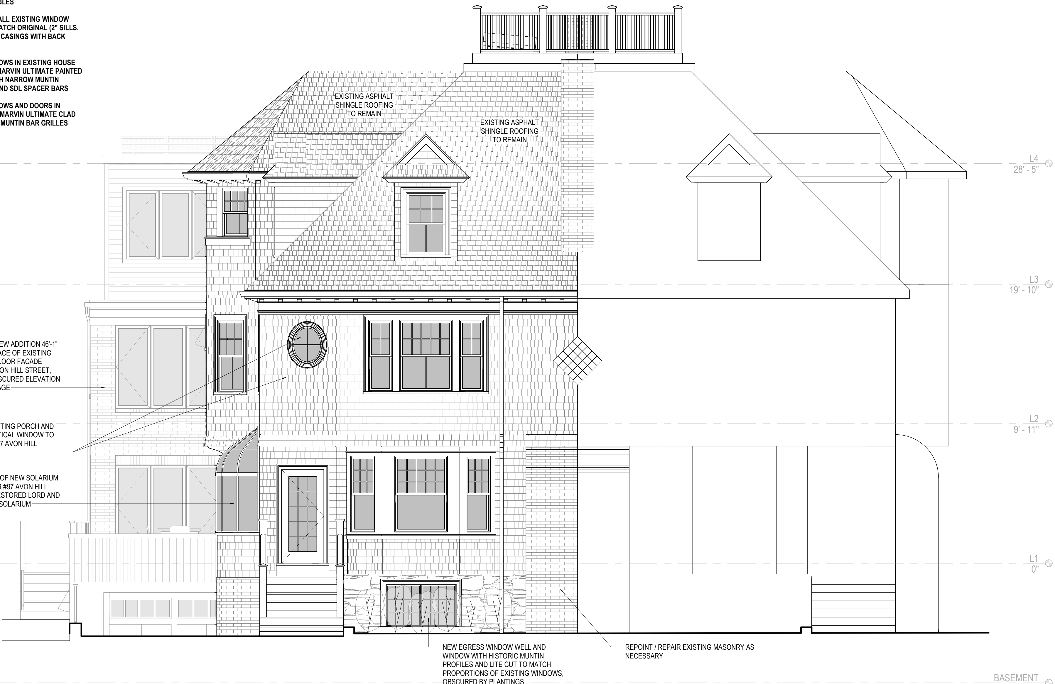
A1 NORTH ELEVATION (AVON HILL STREET) A201 1/4" = 1'-0"
