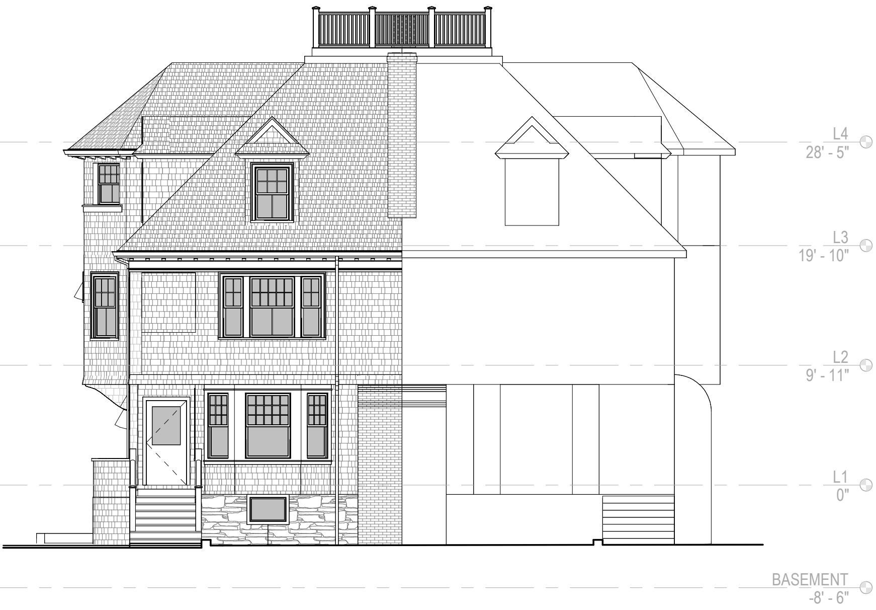
E1 EXISTING NORTH ELEVATION (AVON HILL STREET) A201 1/8" = 1'-0"
