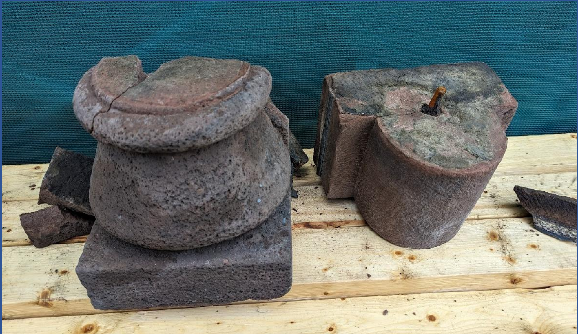
Iron pins and shattered masonry to be replaced
