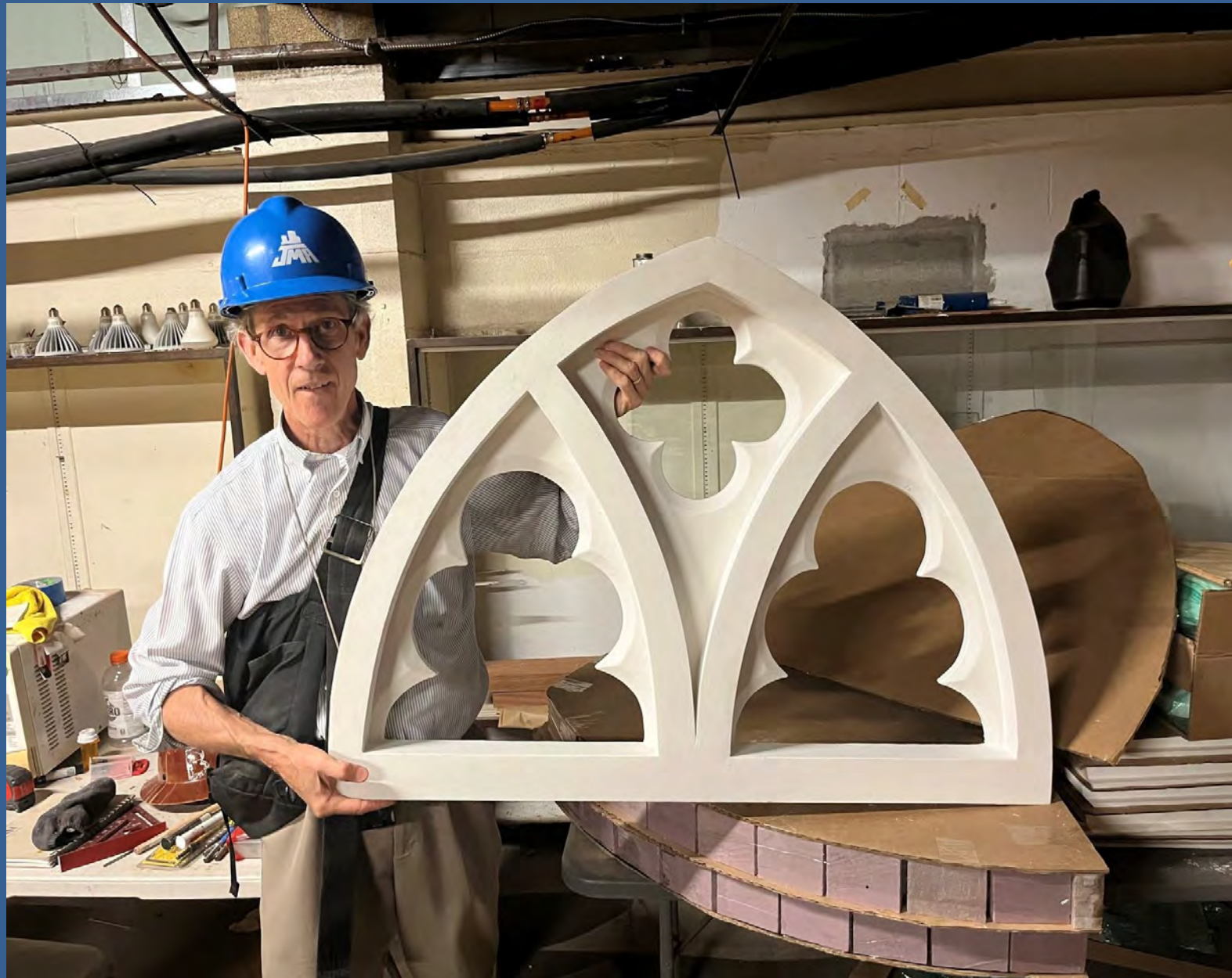
Architect David Torrey with GFRP replacement lancet heads
