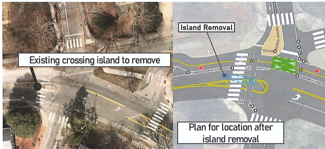
Before and after of crossing island removal
