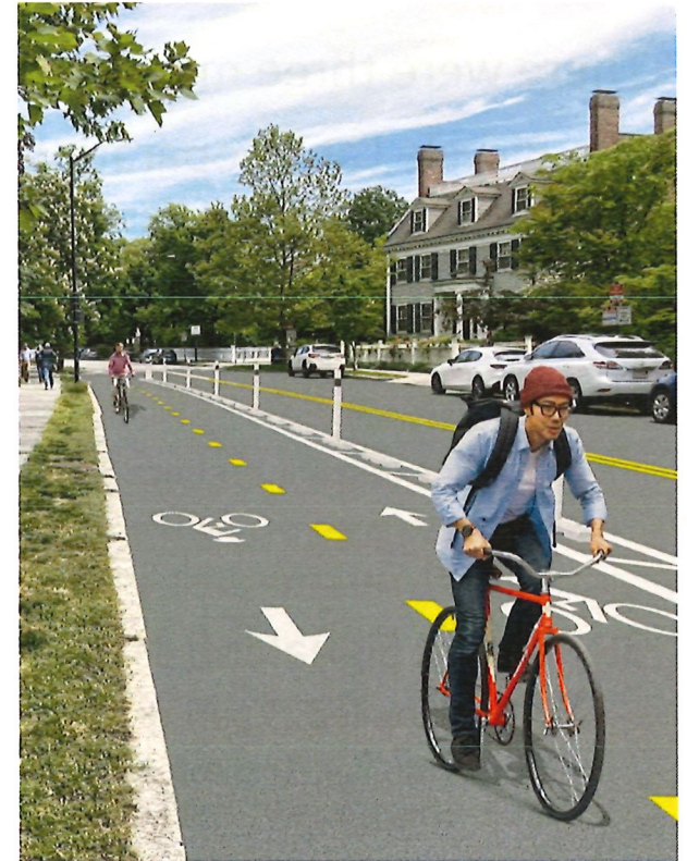
Rendering of Brattle Street using both flexible delineator posts and precast concrete curbing
