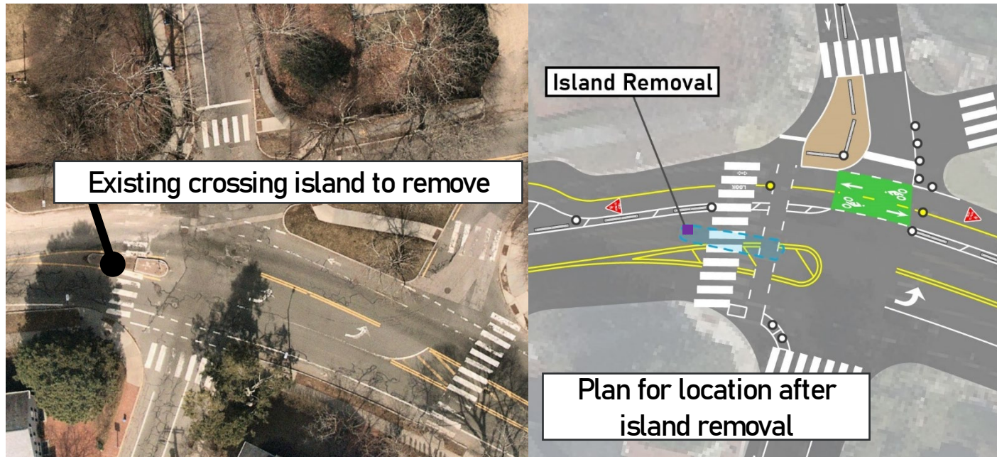
Before and after of crossing island removal
