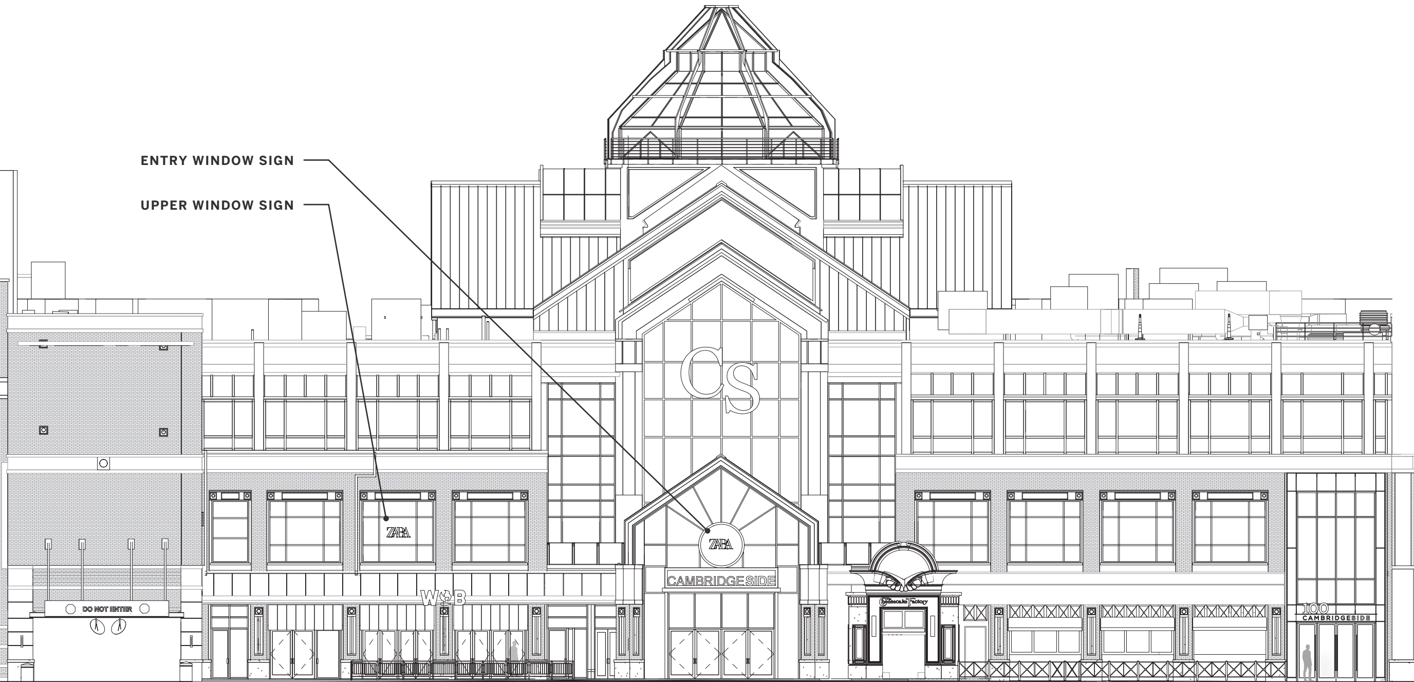
MOUNTING ELEVATION – 100 CAMBRIDGESIDE (SOUTH) SCALE 1/16" = 1'-0"
