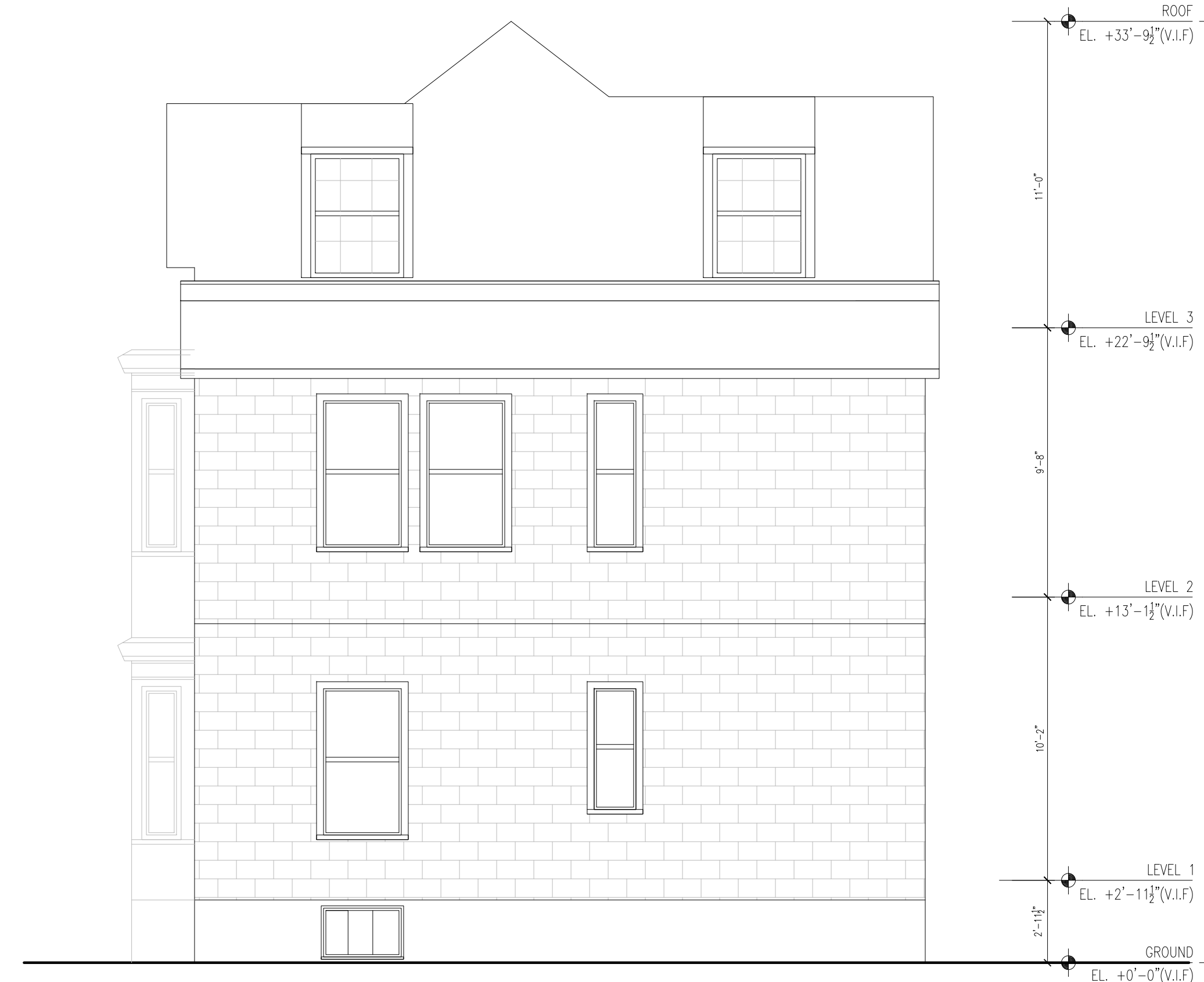
3 EXISTING RIGHT SIDE ELEVATION SCALE: 1/4" = 1'-0"
