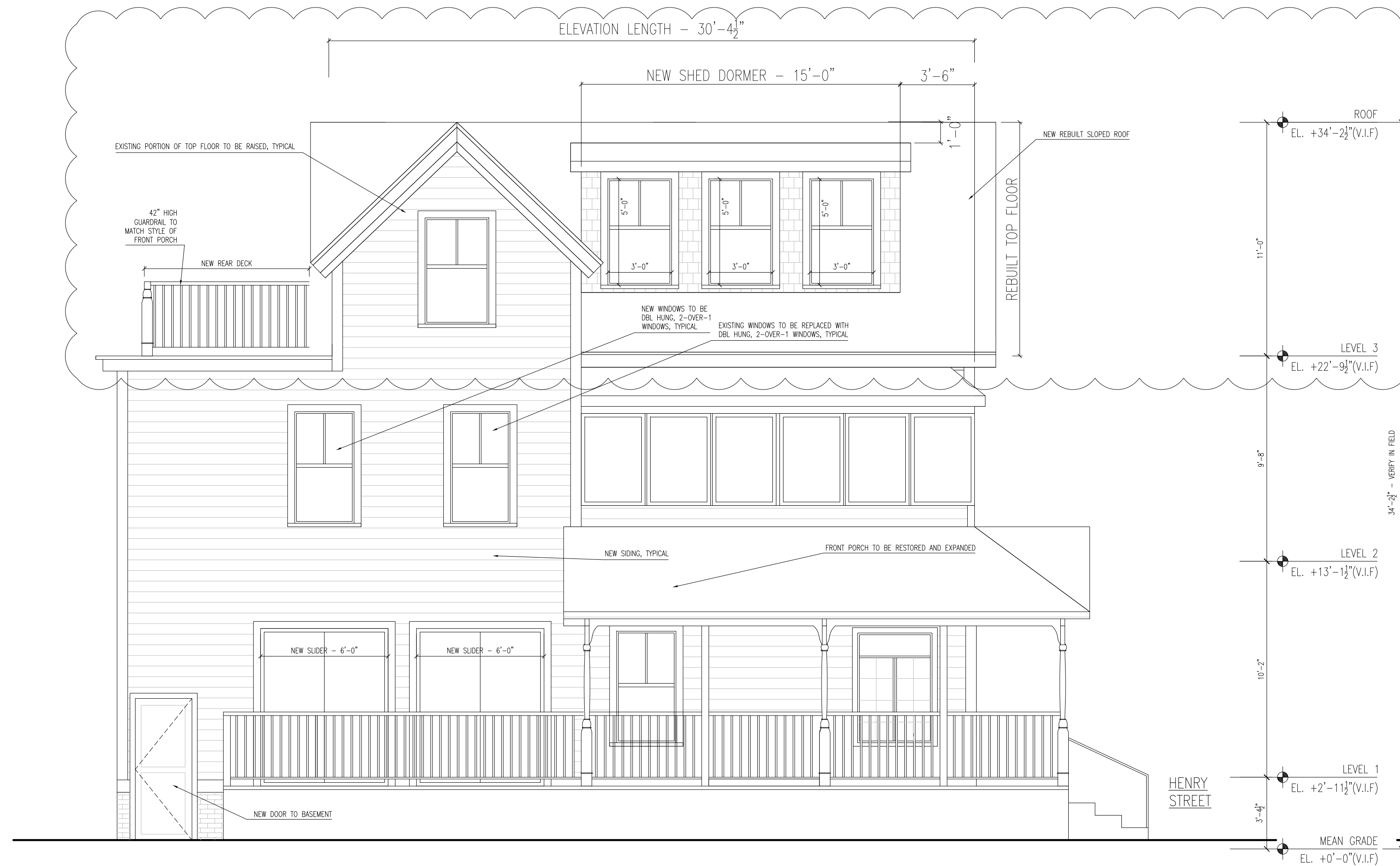
2 PROPOSED LEFT SIDE ELEVATION SCALE: 1/4" = 1'-0"
