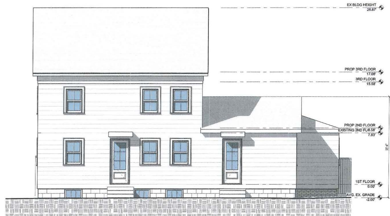
2 EXISTING RIGHT SIDE ELEVATION 1/4" = 1'-0"
