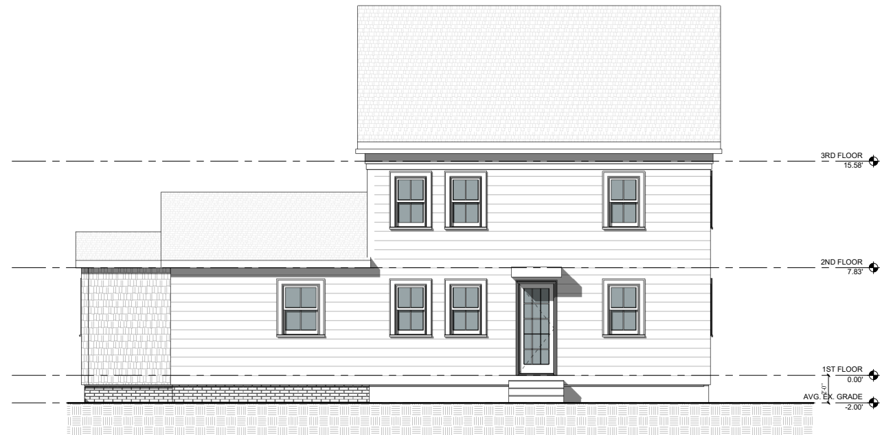
② EXISTING LEFT SIDE ELEVATION 1/4" = 1'-0"
