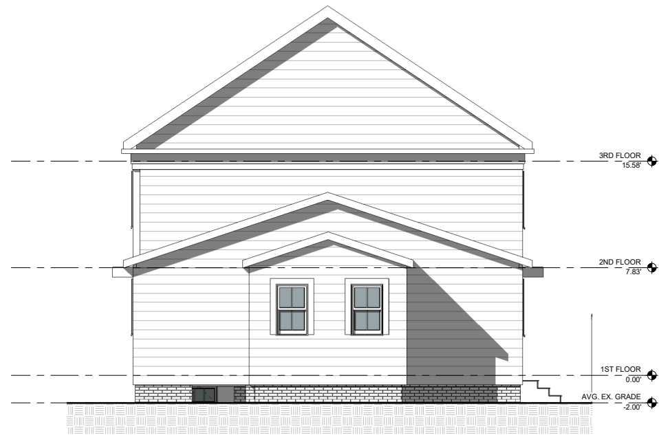
③ EXISTING REAR ELEVATION 1/4" = 1'-0"
