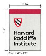
Materials: Powder coated graphic panel with 3/4\* thick fabricated aluminum frame painted black and mounted to fence.
