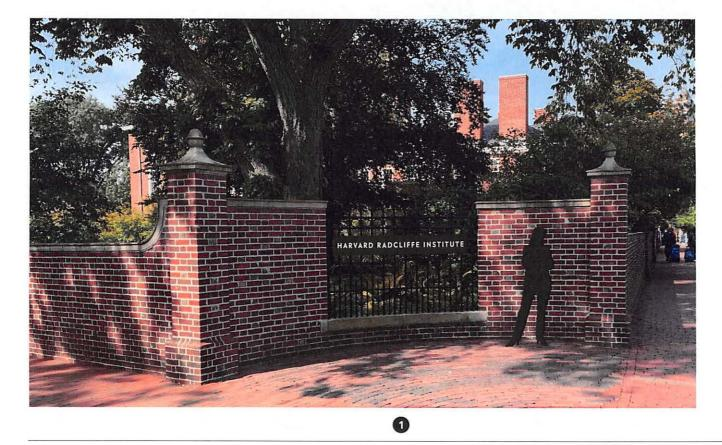
Materials: 1/4\* thick painted aluminum panel with 3/16\* thick painted aluminum letters mounted to existing iron fence with no visible fasteners.
