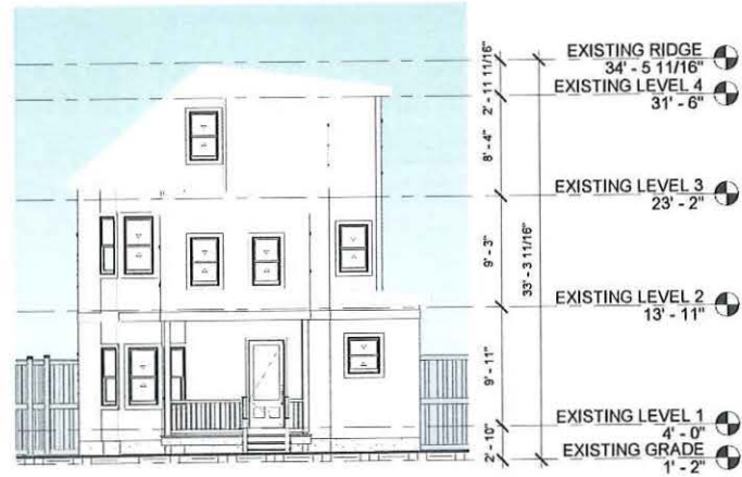
1 BZA - EXISTING SOUTH ELEVATION 1/8" = 1'-0"
