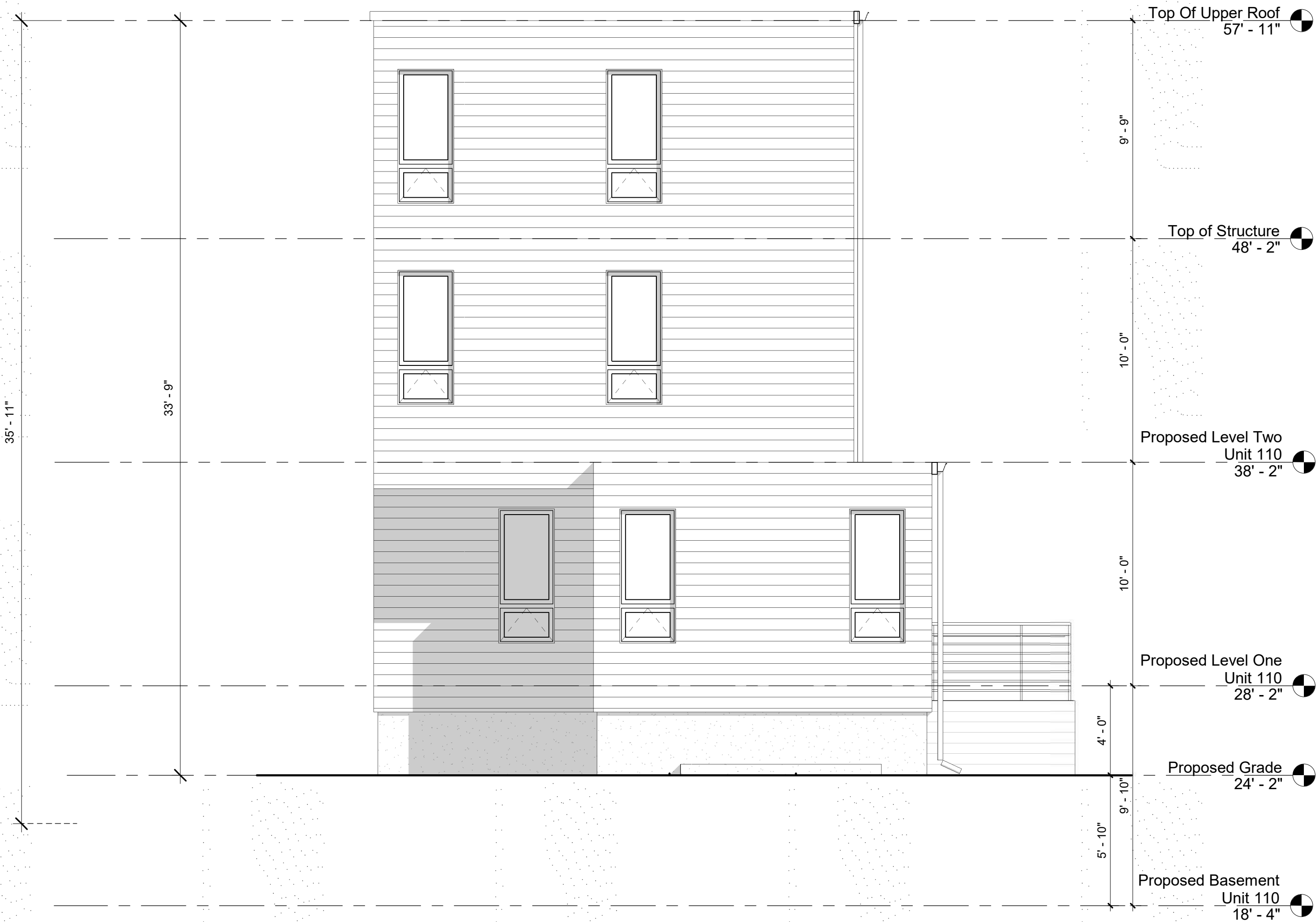
④ Proposed Right Elevation Unit 110 1/4" = 1'-0"
