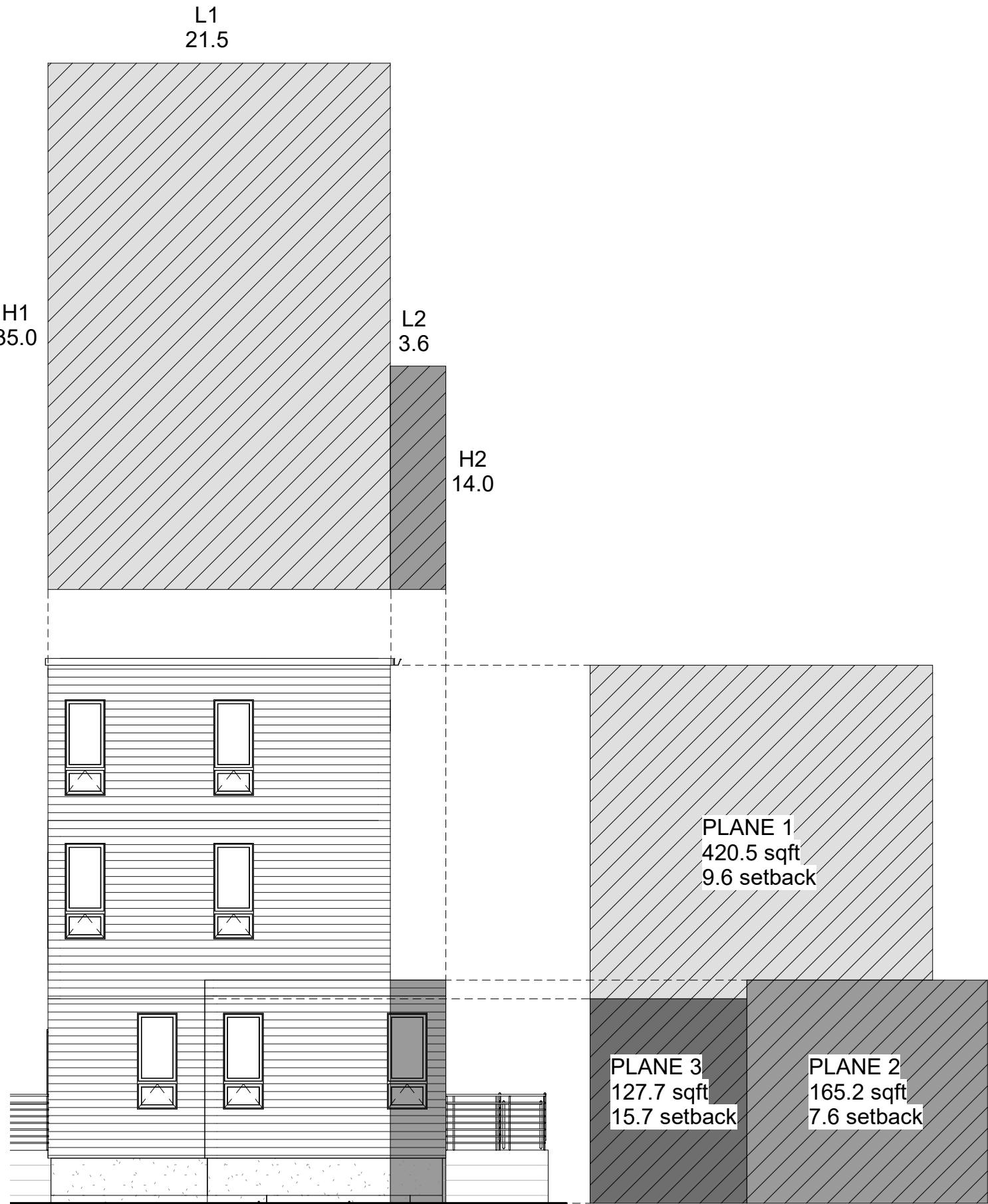
2 Proposed Right Elevation Unit 110 Setback 1/8" = 1'-0"
