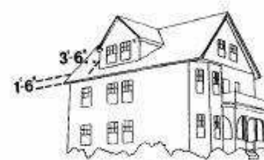
Figure 11: If the gable dormer meets the recommended setbacks for side (3 ft. 6 in.) and front (1 ft. 6 in.) walls, the dormer roof may extend from the ridge line.
