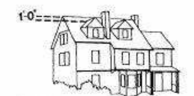
Figure 12: Gable dormers added in combination, such as pairs, should not exceed 15 ft. in total length. The preferred setback from the roof ridge should be at least 1 foot.
