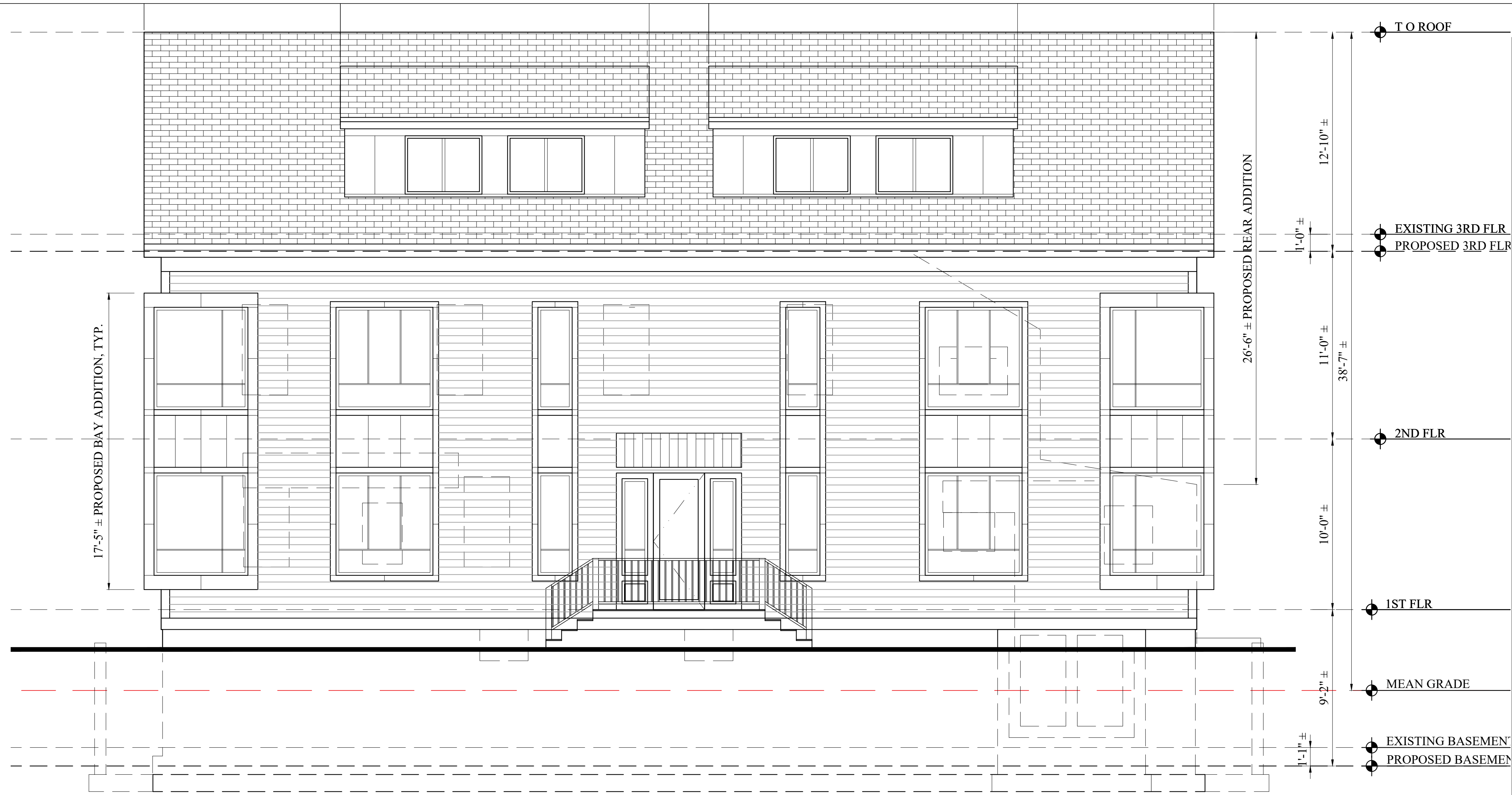
2 PROPOSED SIDE ELEVATION 1/4" = 1'-0"
