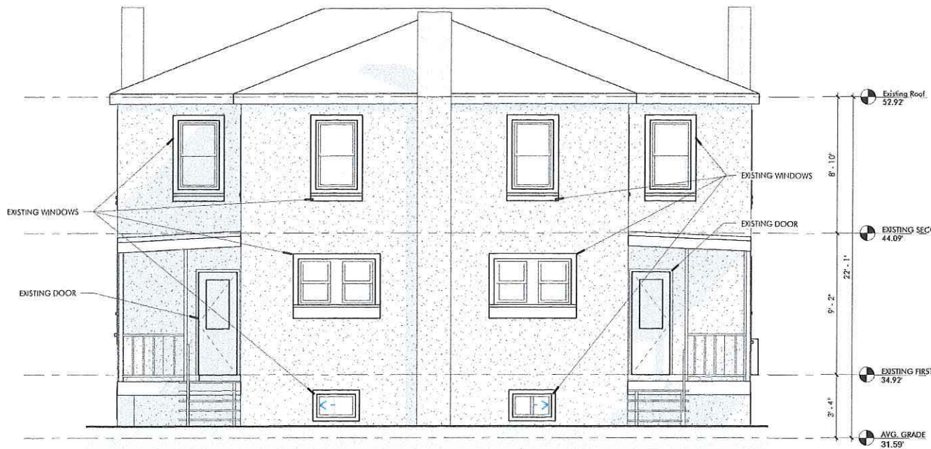
② EXISTING WEST ELEVATION 1/4" = 1'-0"
