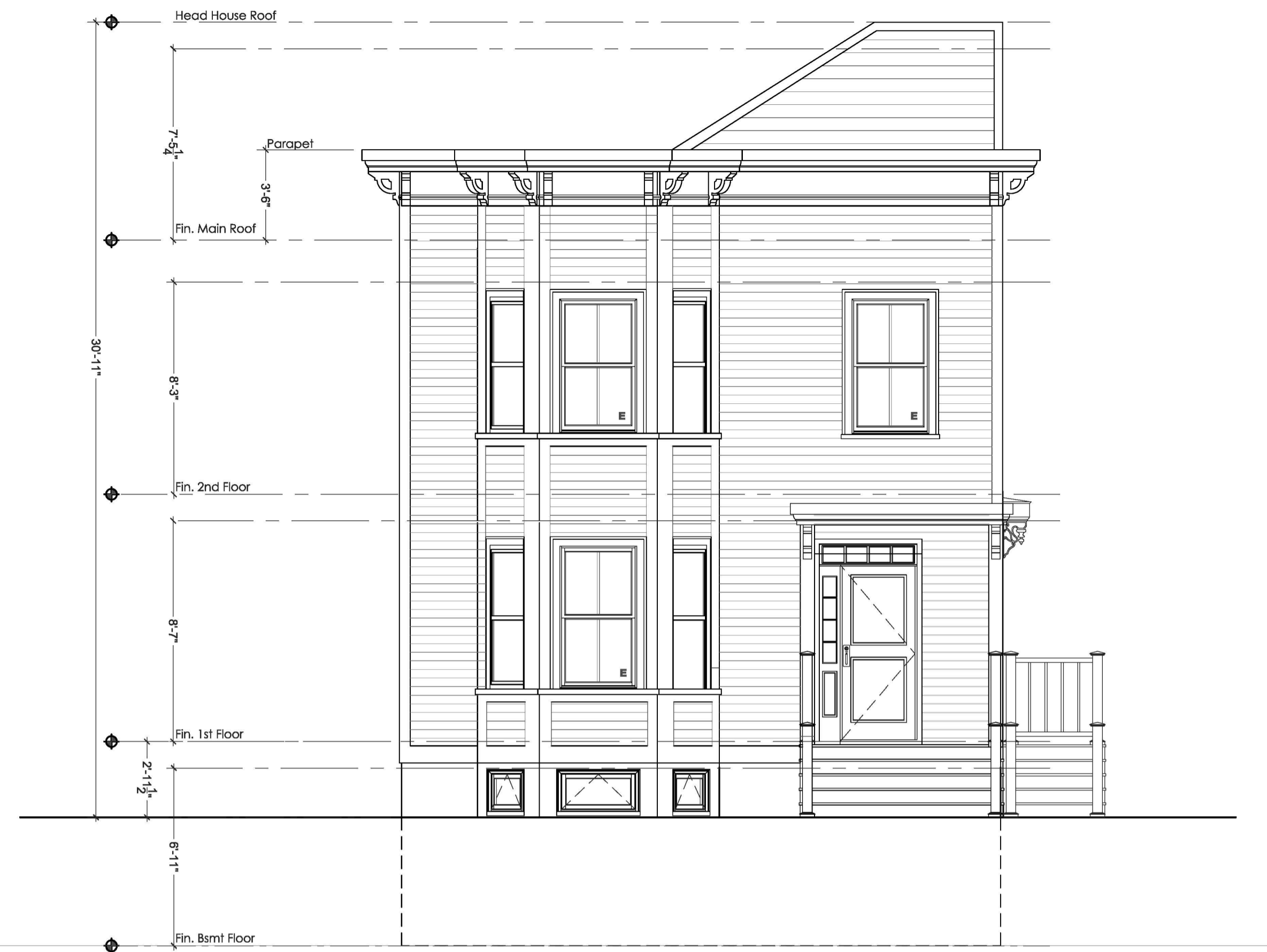
② EXISTING EAST ELEVATION Scale: 1/4" = 1'-0"
