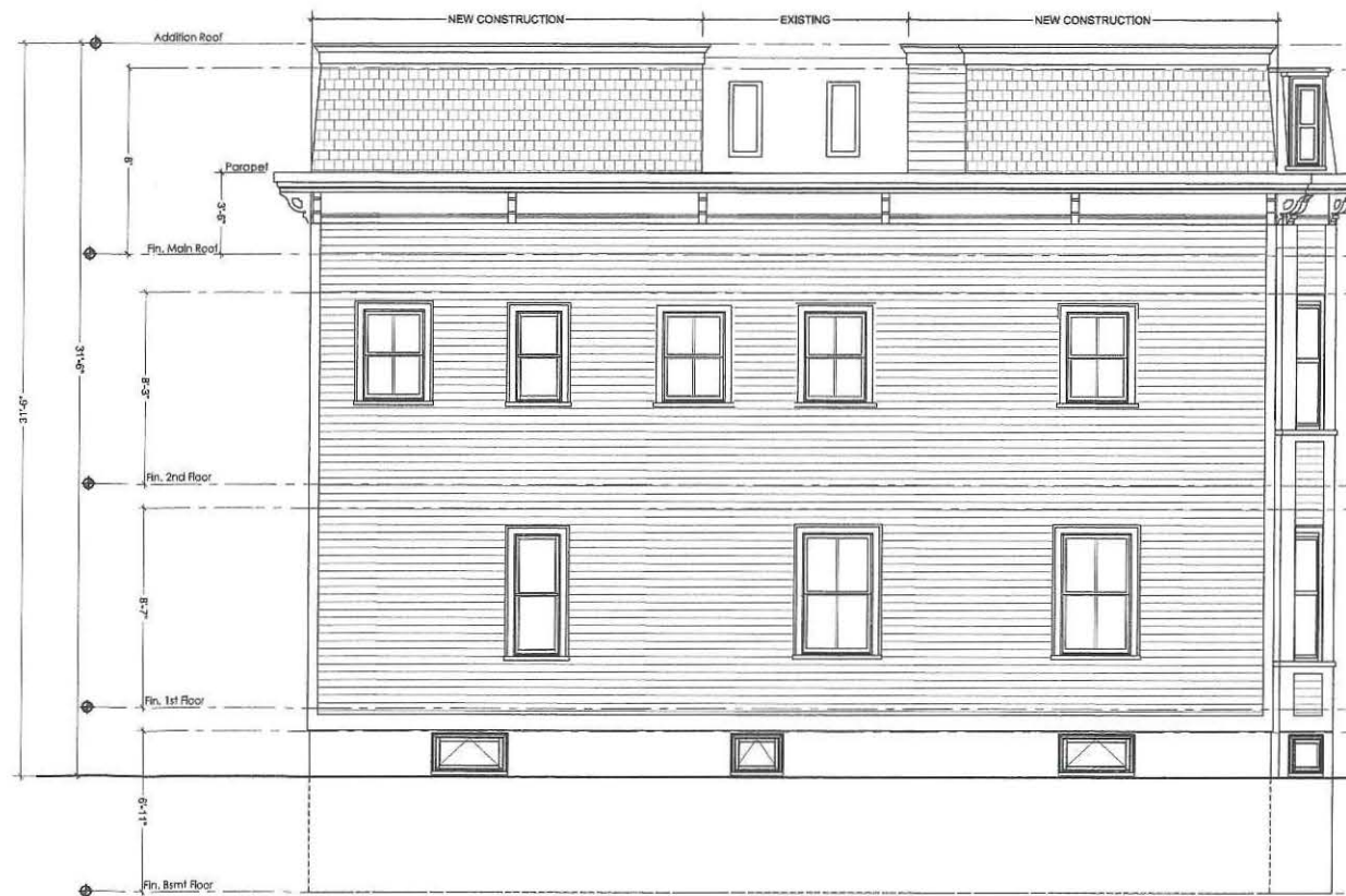
④ PROPOSED SOUTH ELEVATION Scale: 1/4" = 1'-0"
