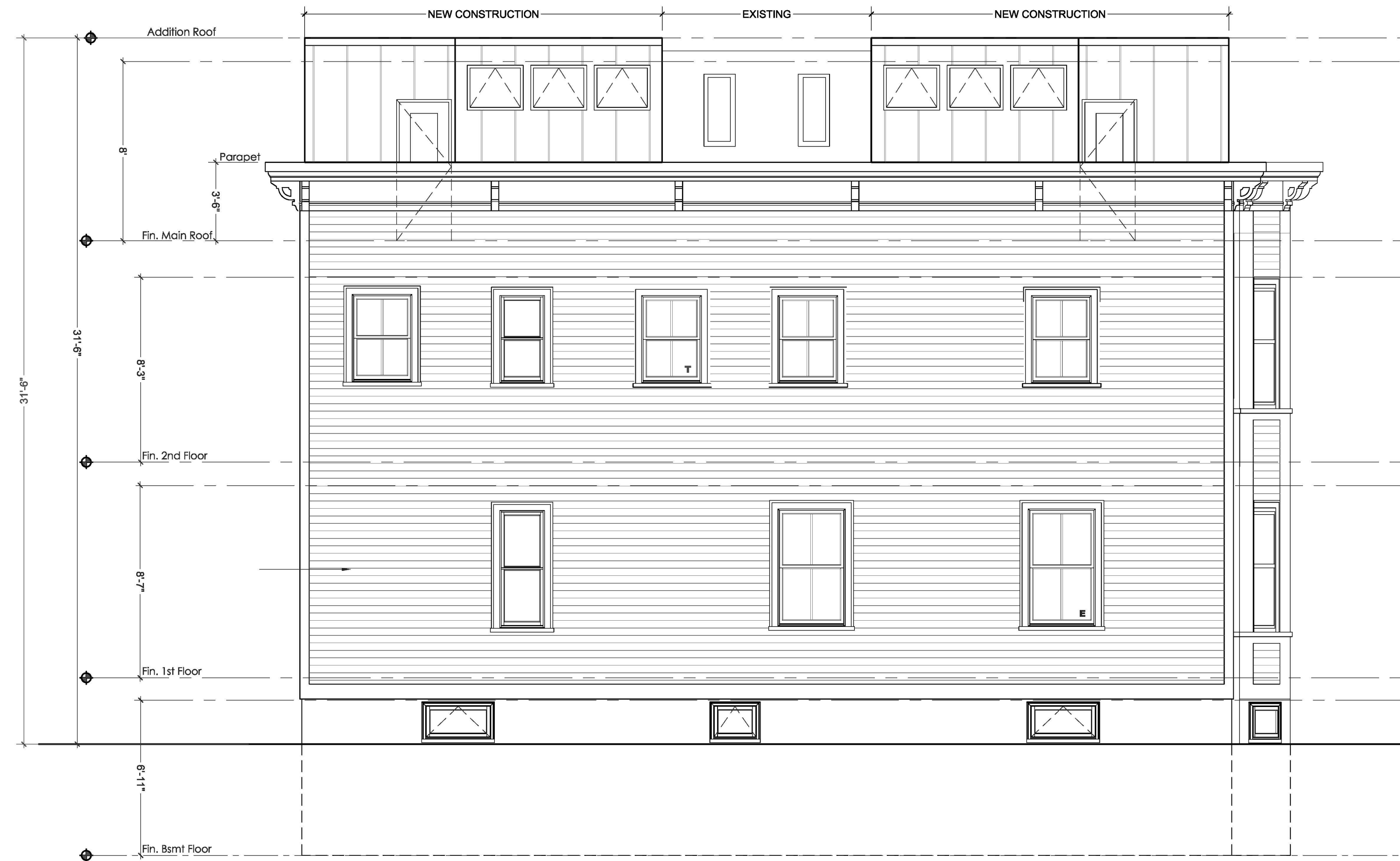
④ PROPOSED SOUTH ELEVATION Scale: 1/4" = 1'-0"
