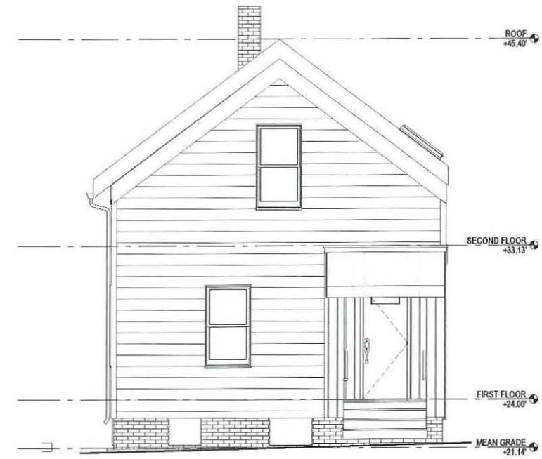
2 EAST ELEVATION - EXISTING SCALE: 1/4" = 1'-0"
