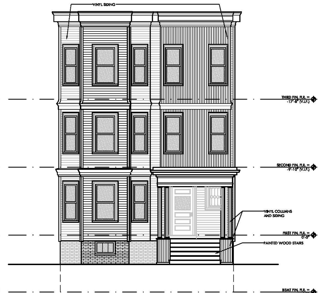
2 EXISTING NORTH ELEVATION 1/8" = 1'-0"
