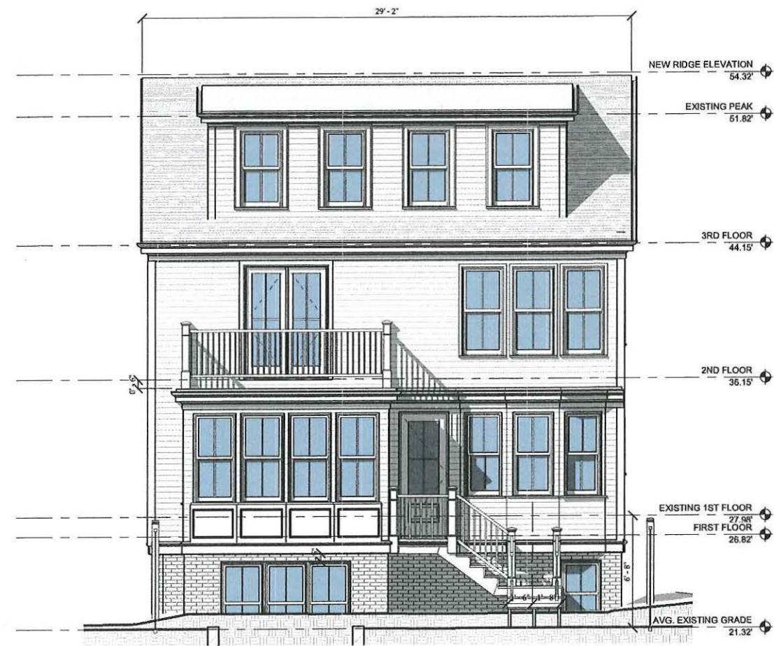
① FRONT ELEVATION - PROPOSED 1/4" = 1'-0"
