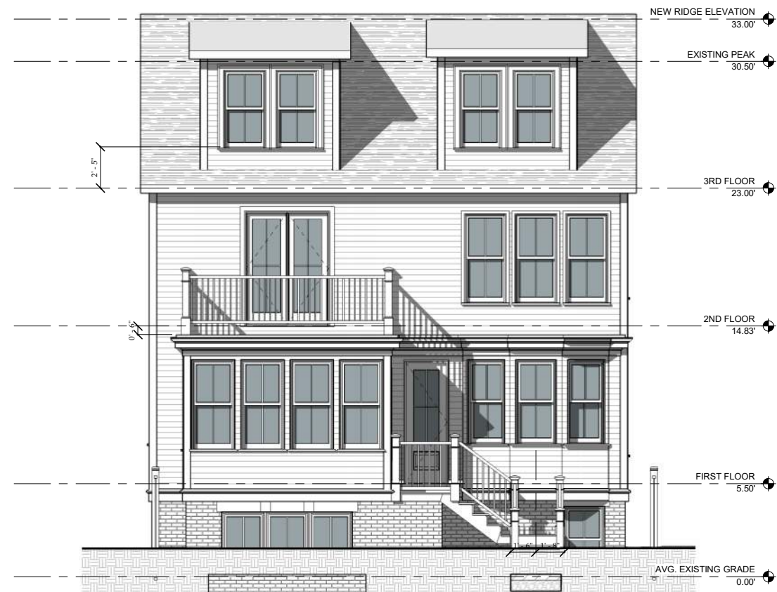
① FRONT ELEVATION - ALTERNATE 1/4" = 1'-0"
