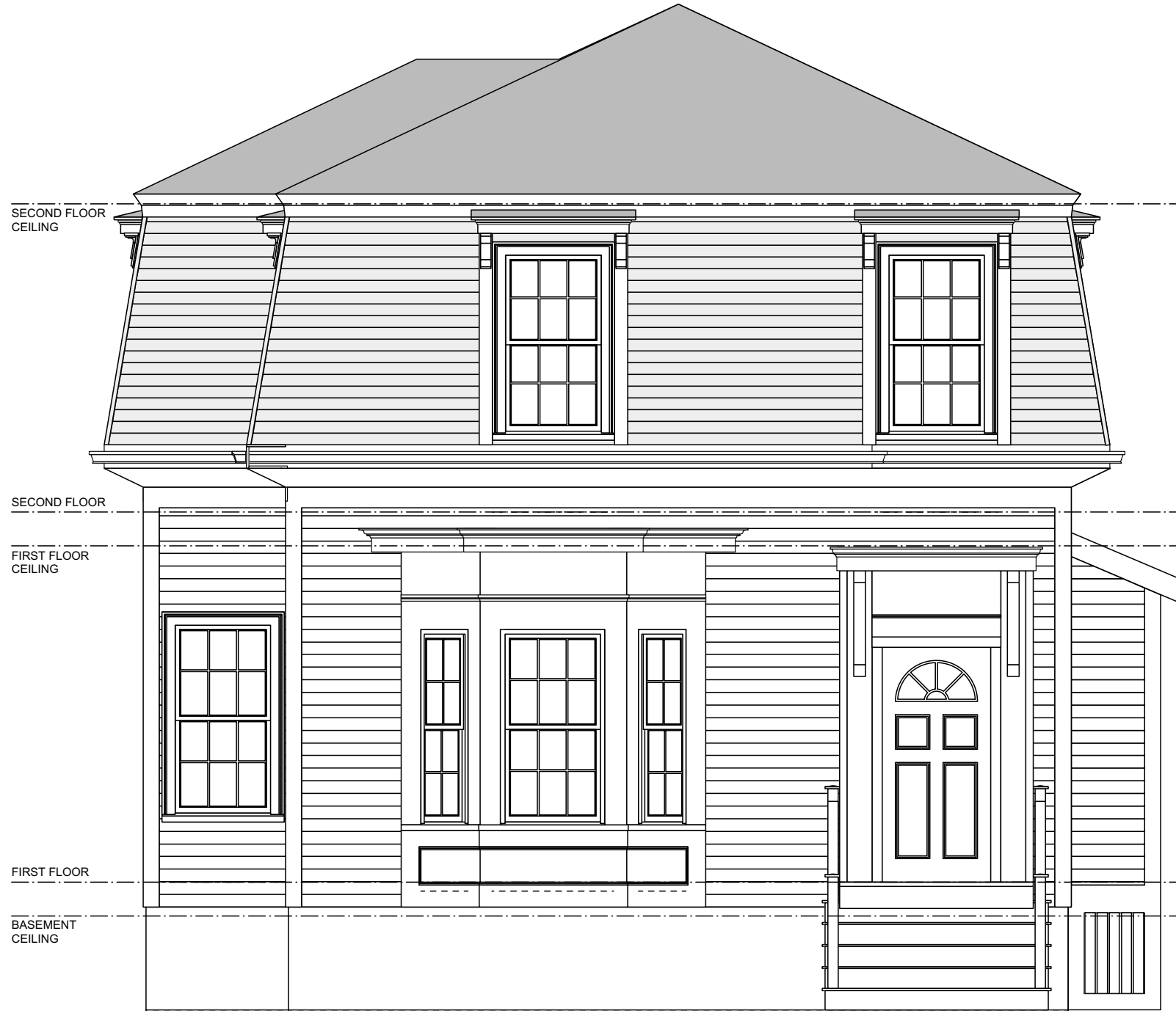
EXISTING FRONT ELEVATION 1/4" = 1'-0" 0 5 FT
