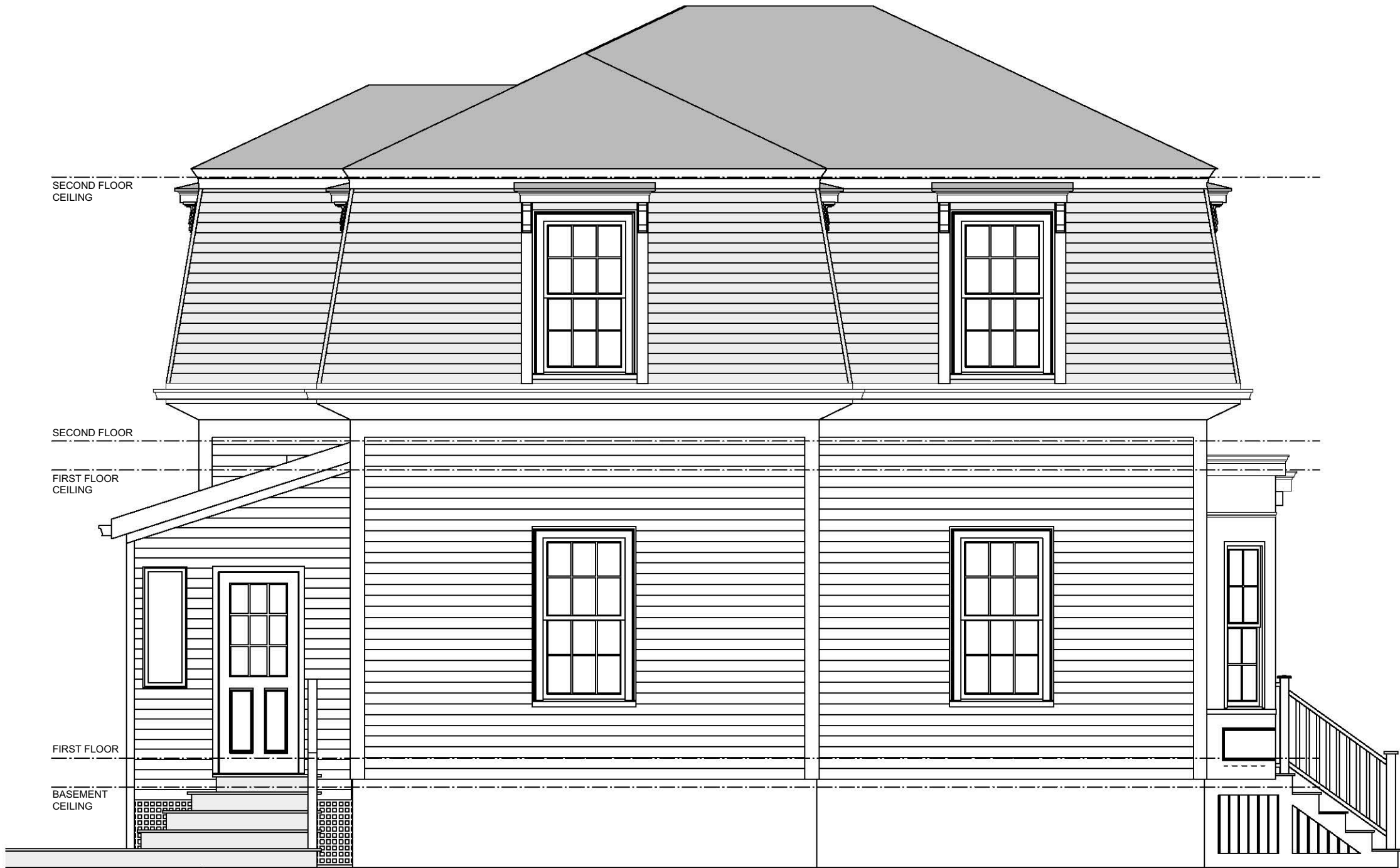
PROPOSED LEFT SIDE ELEVATION 1/4" = 1'-0" 0 5 FT
