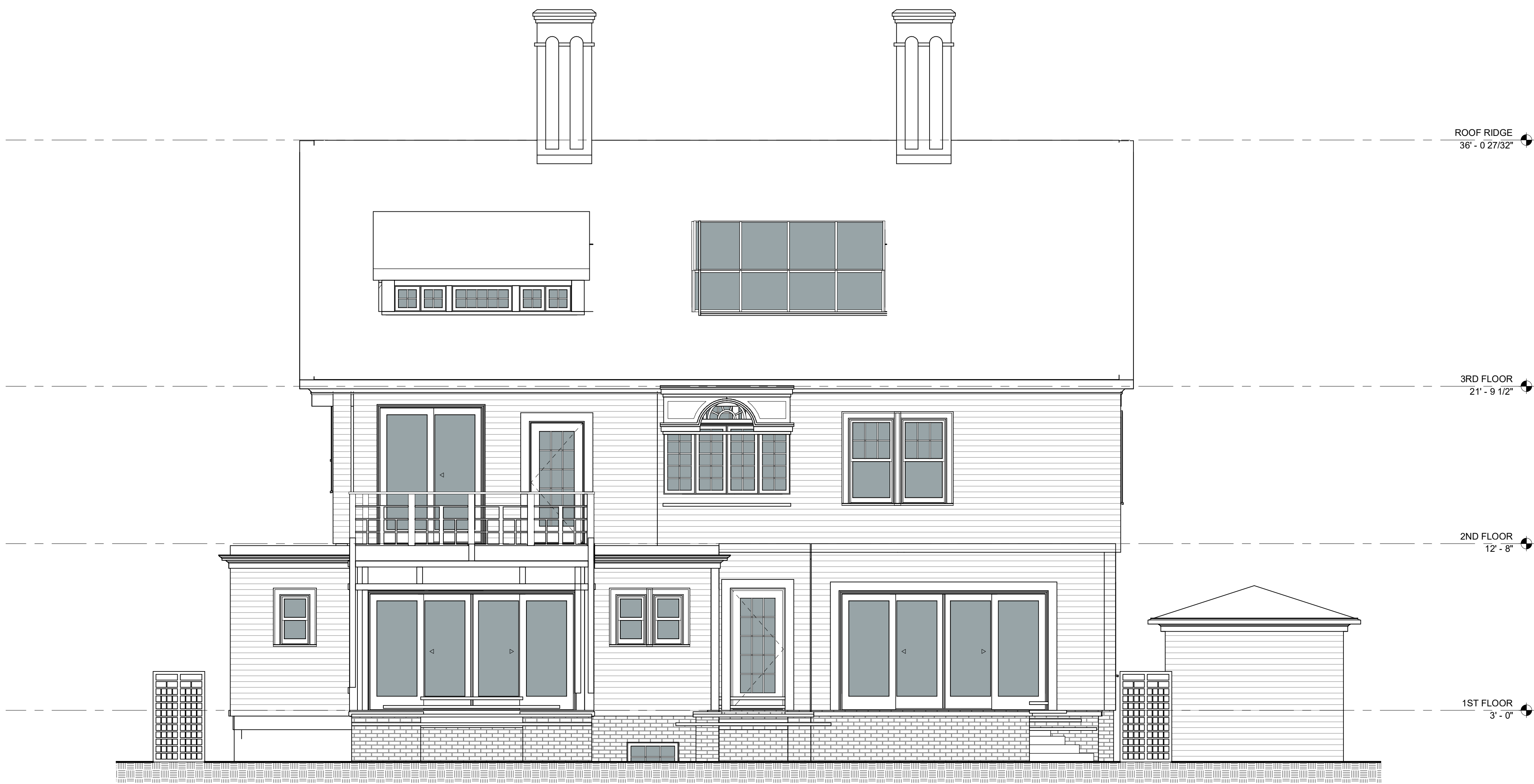
1 EXISTING ELEVATION - REAR 1/4" = 1'-0"
