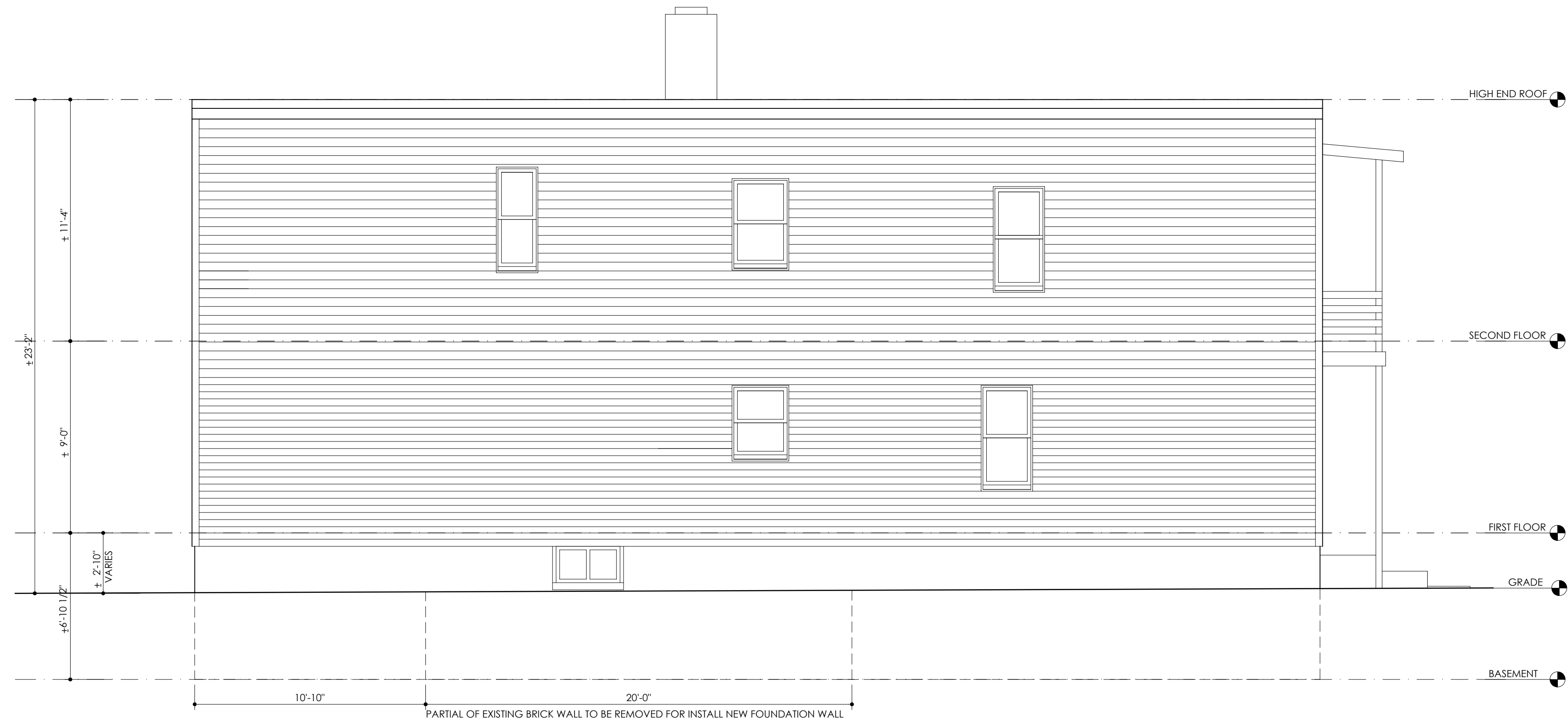
2 EXISTING/DEMOLITION RIGHT SIDE ELEVATION A1.1 1/4"=1'-0"
