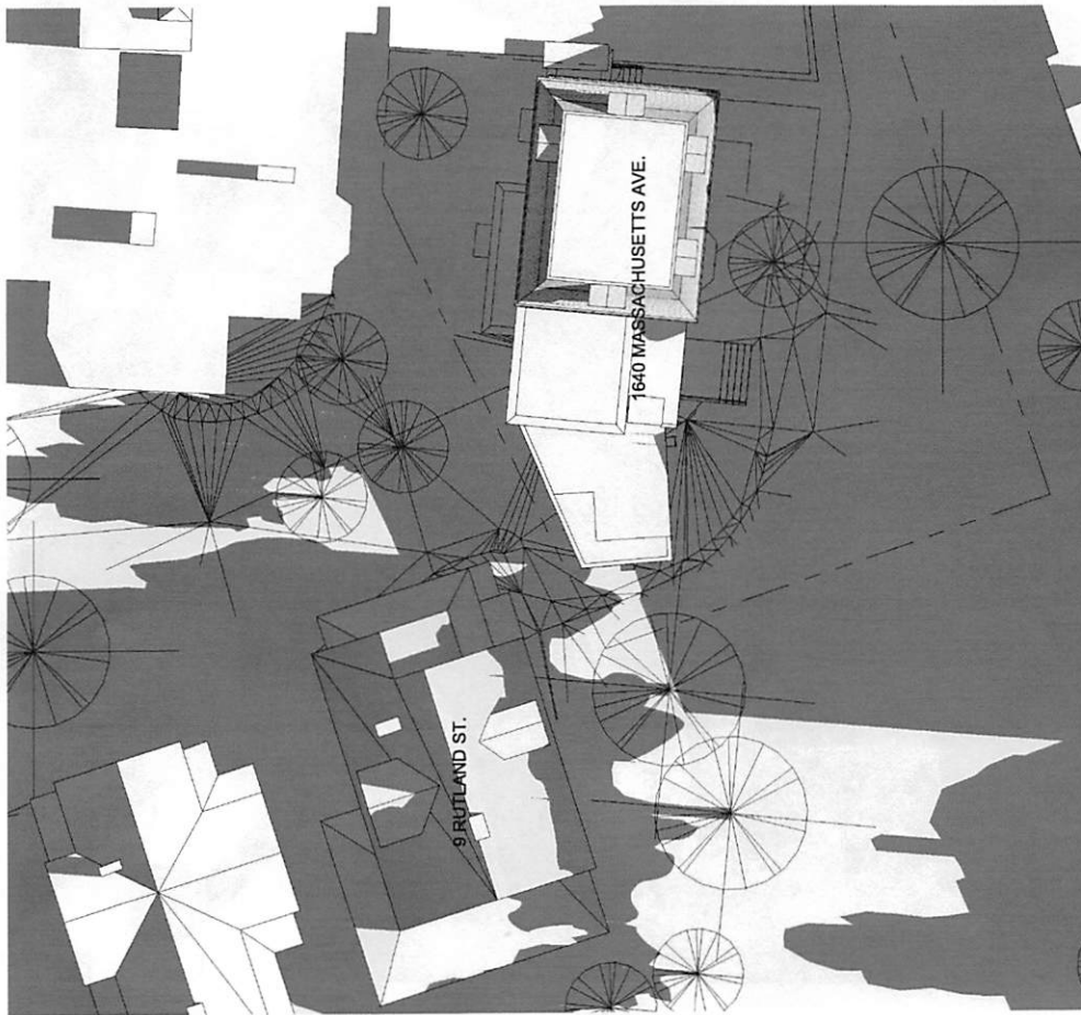
① Existing Solar Study - Dec 21st - 12 PM 1" = 20'-0"
