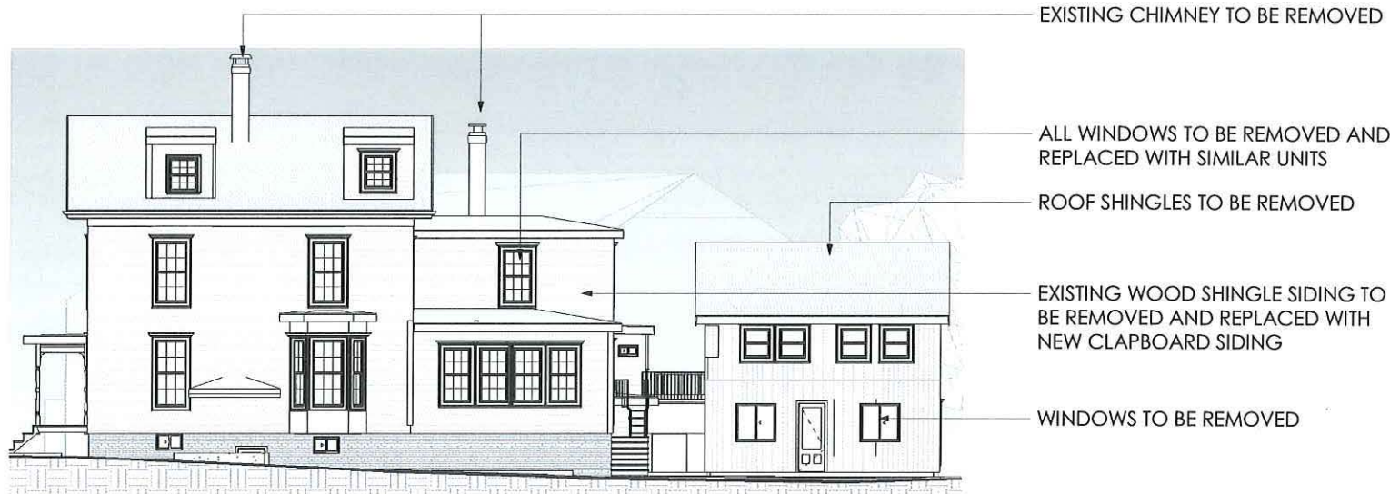
1 EXISTING - SOUTH ELEVATION - Dependent 1 1/8" = 1'-0"
