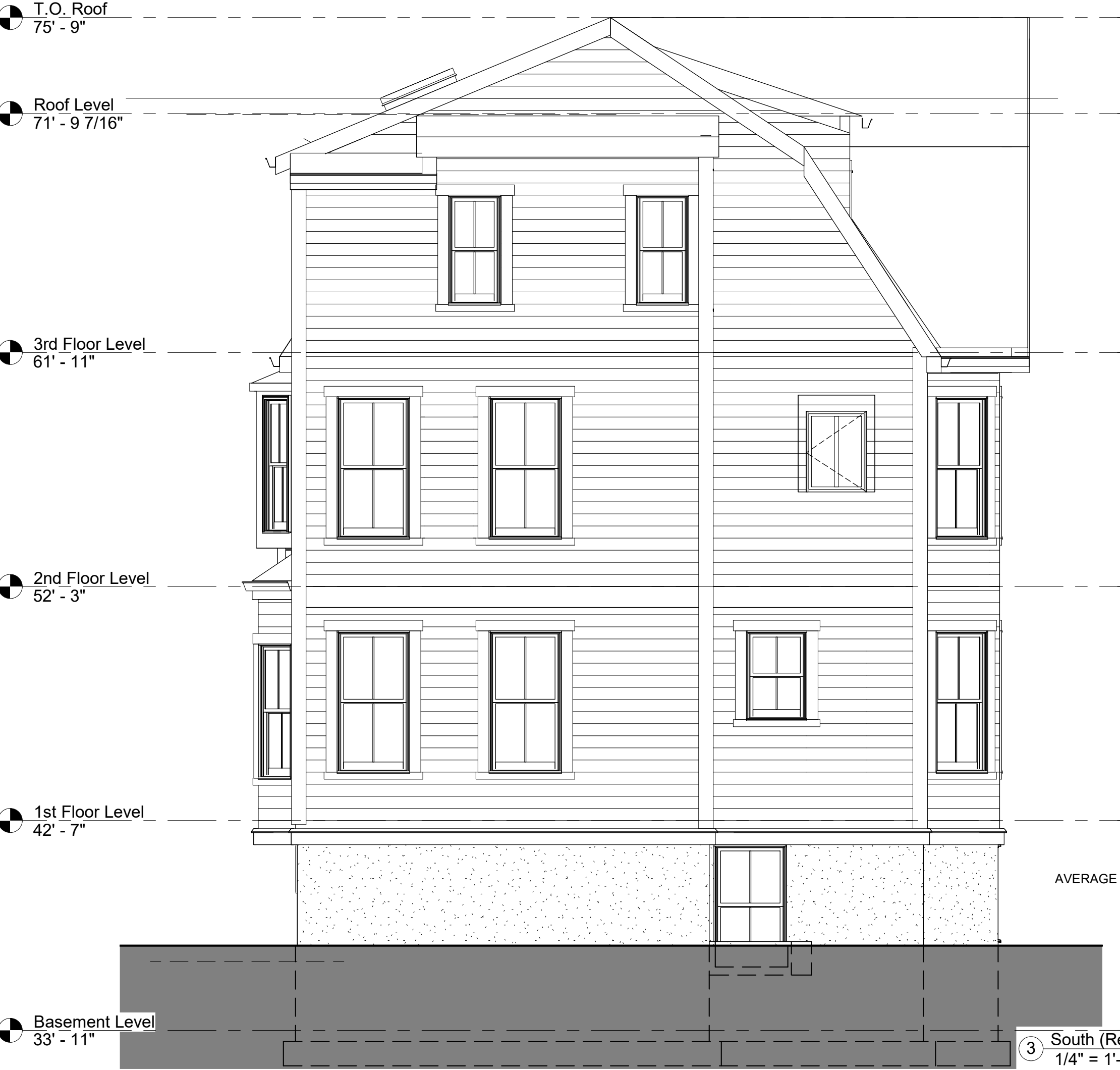
1 North (Front) Elevation 1/4" = 1'-0"
