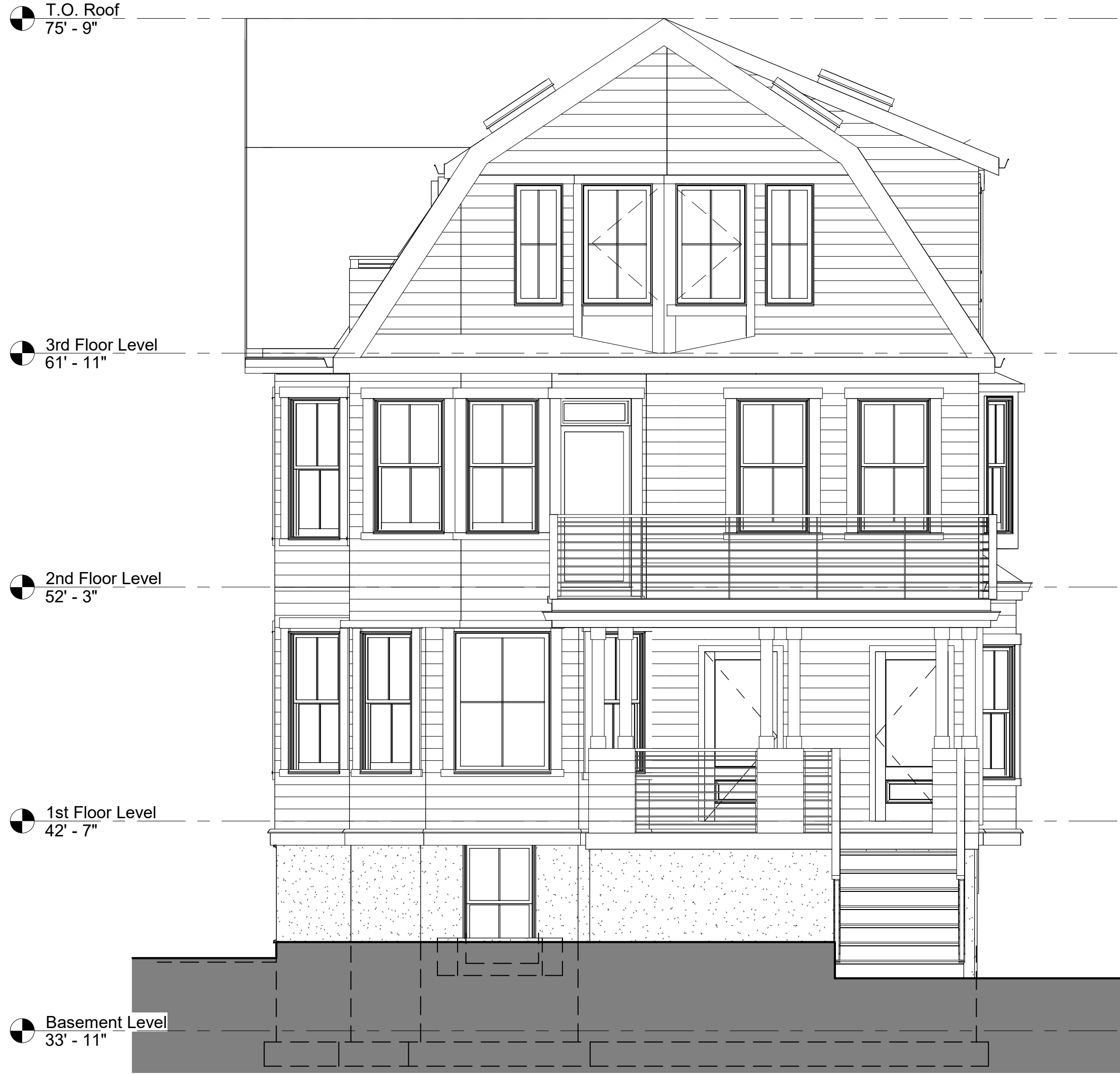
1 North (Front) Elevation 1/4" = 1'-0"
