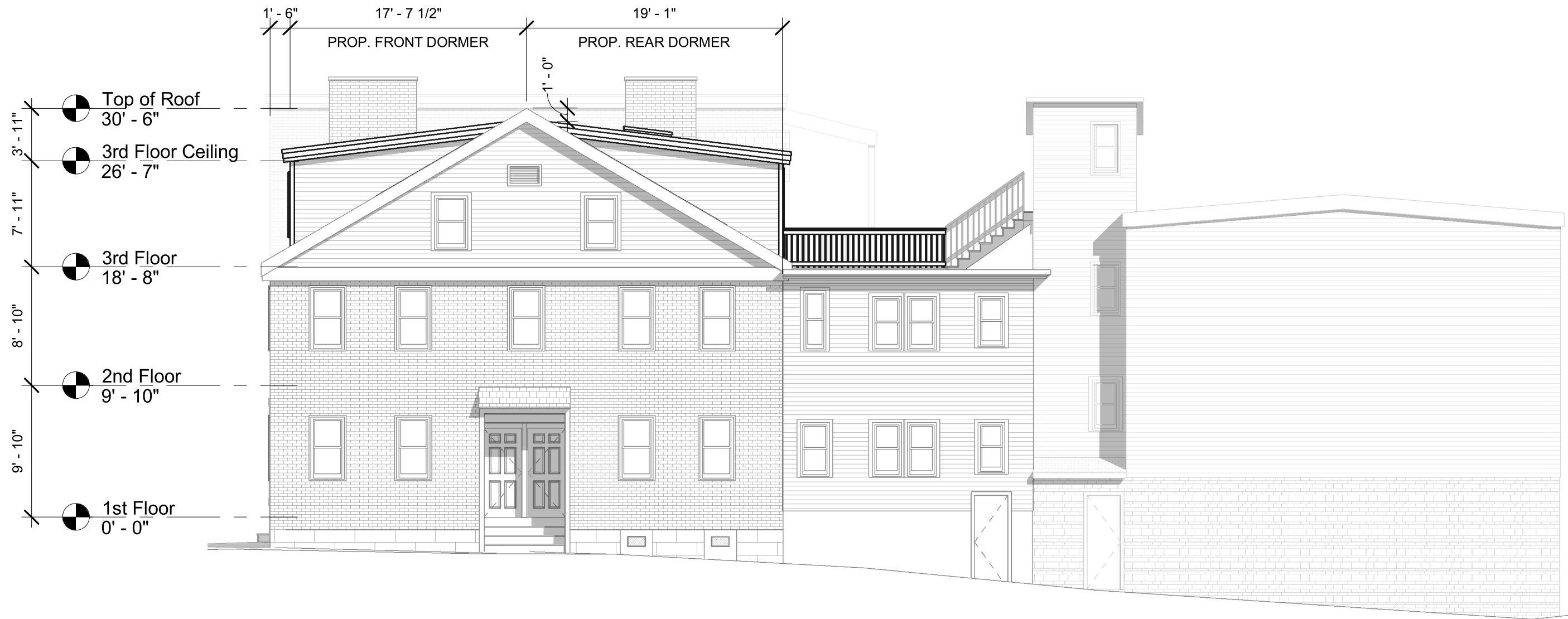
① Prop. Front Elevation - Third Street 1/8" = 1'-0"
