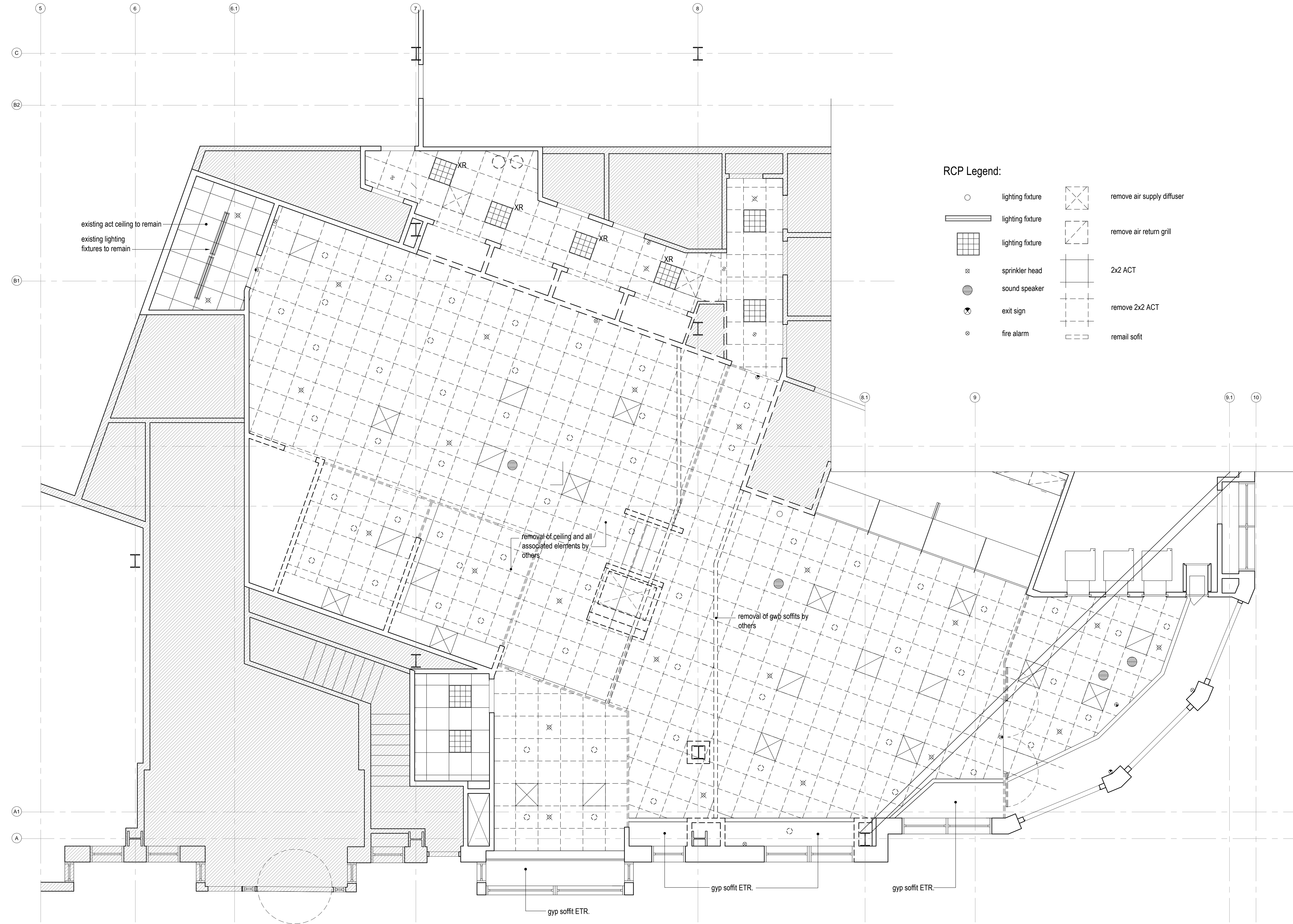
1 Demolition Reflected Ceiling Plan
