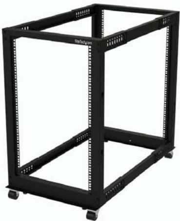
MANUFACTURER: STAR TECH OR EQUIVALENT MODEL: 18U 19" OPEN FRAME SERVER RACK DIMENSIONS (HxWxD): 35.6"x23.6"x22"-40" WEIGHT: 65 LBS.
