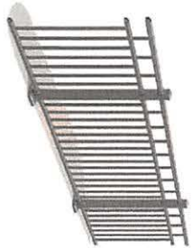
3 TYPICAL SECTION AT ALUMINUM BALUNING ASSEMBLY SCALE: 1/4" = 1'-0" ALUMINUM BALUNING ASSEMBLY BY VEIN MANNING CO. AND 1/2" x 1/2" x 1/2" ALUMINUM CORNER COUPLER TO PROTECT AT DECK EDGE. SYSTEM SHALL BE INSTALLED IN ACCORDANCE WITH MANUFACTURER'S INSTALLATION INSTRUCTIONS.
