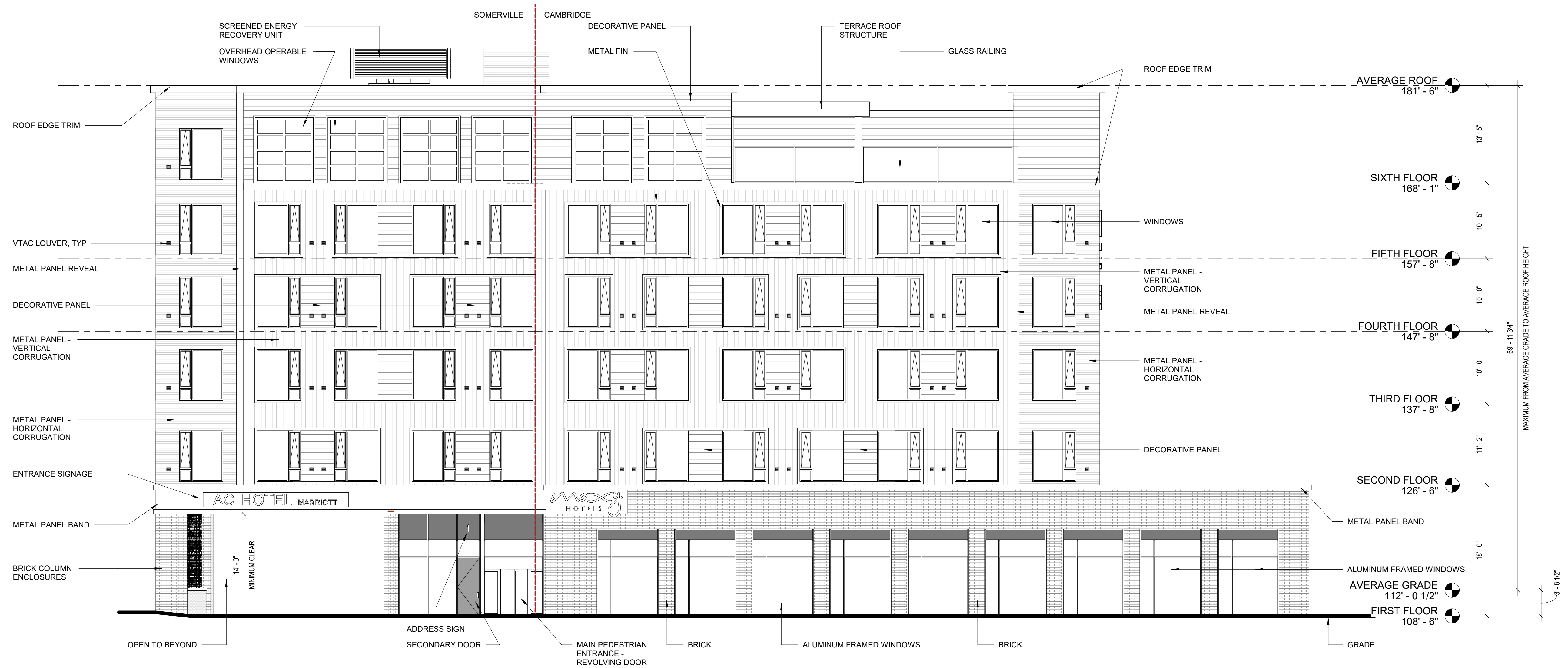
1 EXTERIOR ELEVATION - SOUTH 1/8" = 1'-0"
