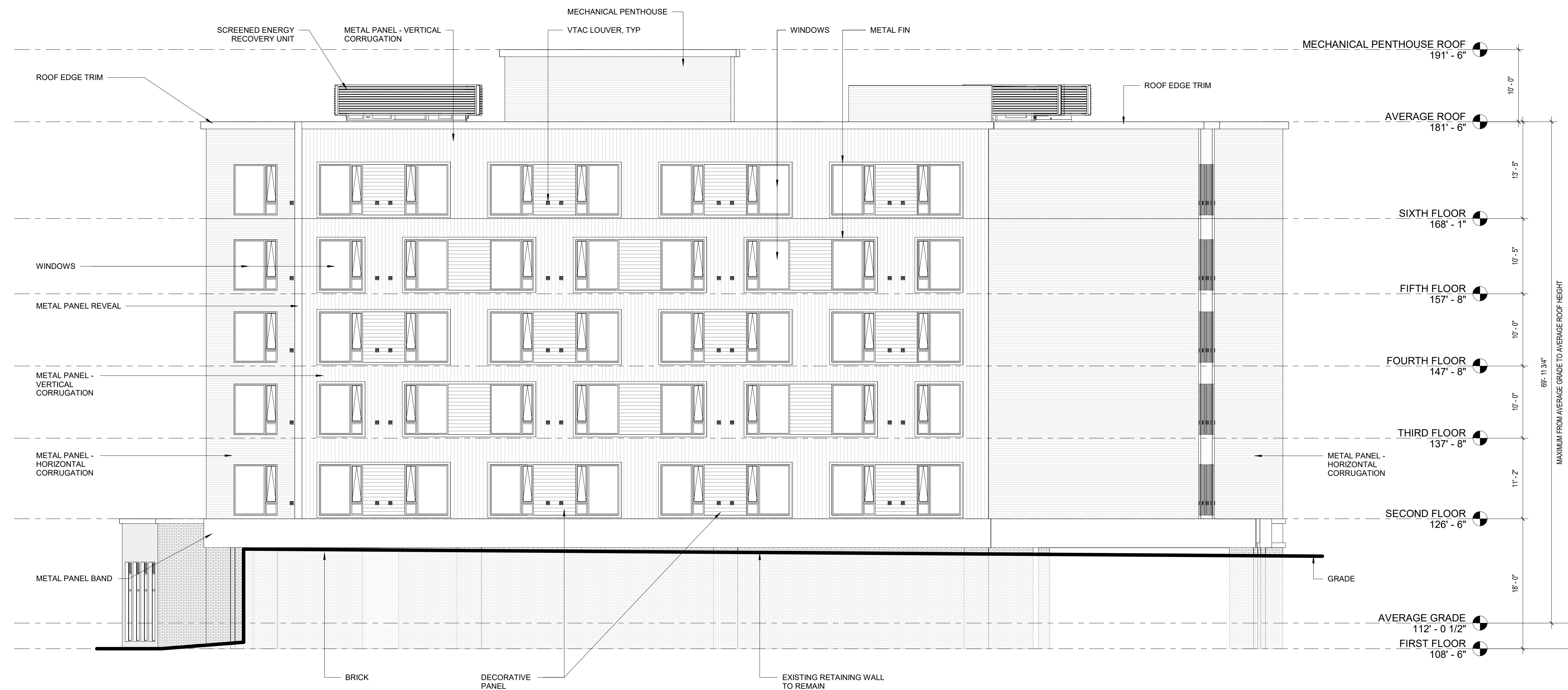
1 EXTERIOR ELEVATION - NORTH 1/8" = 1'-0"
