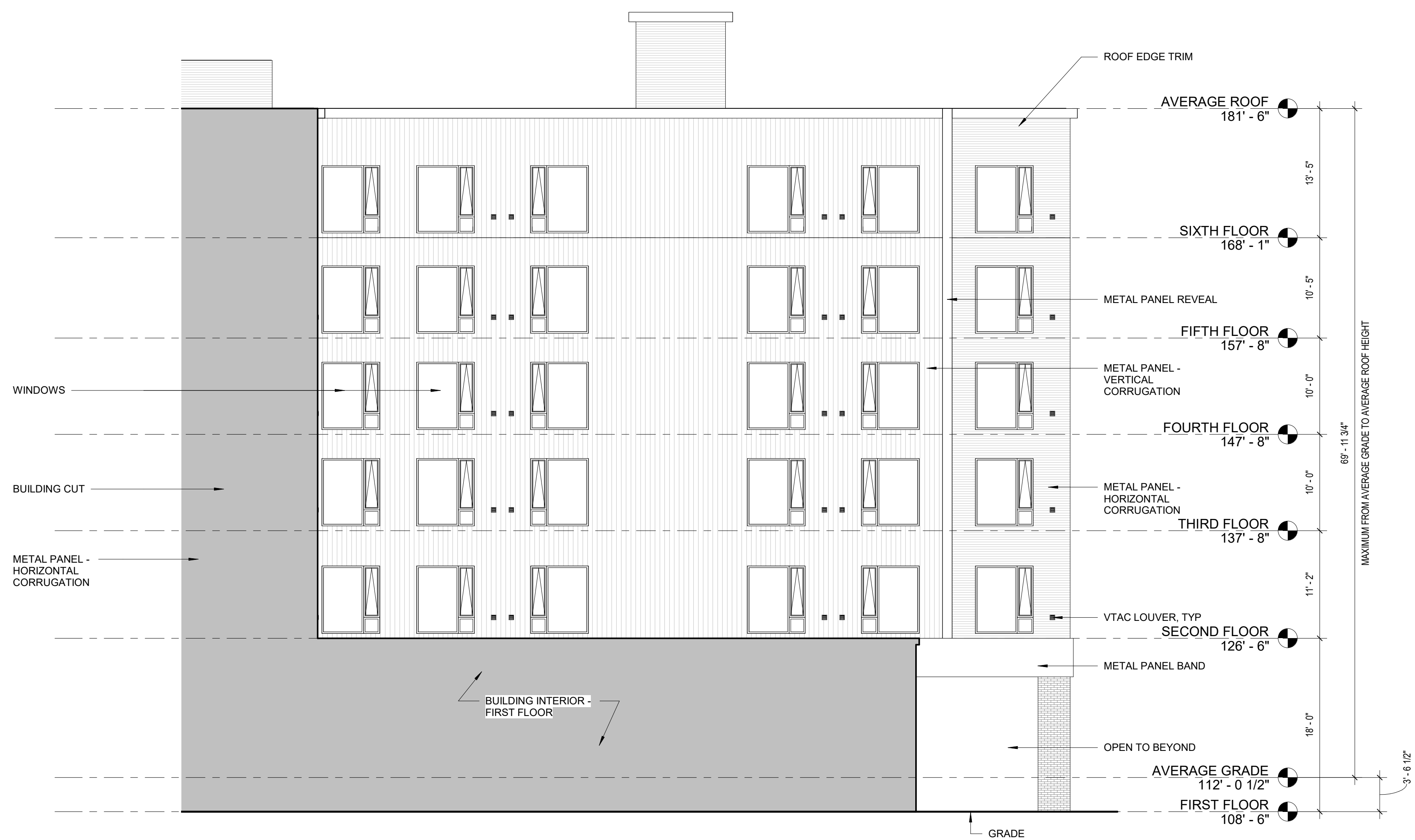
1 EXTERIOR ELEVATION - COURTYARD NORTH 1/8" = 1'-0"
