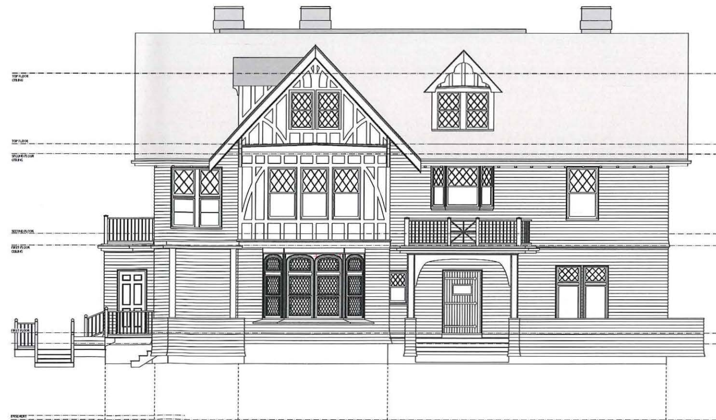
EXISTING FRONT ELEVATION 3/16" = 1' 0" 10 FT
