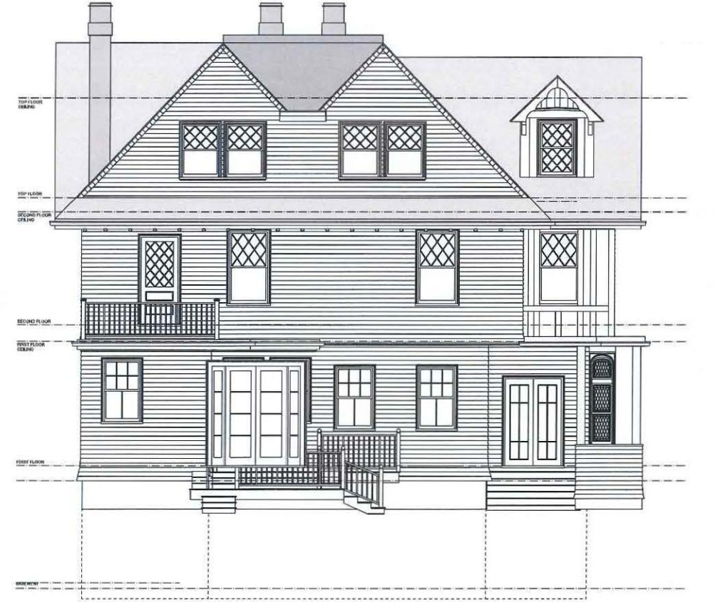
EXISTING REAR ELEVATION (WEST) 3/16" = 1'-0" 0 5 10 FT
