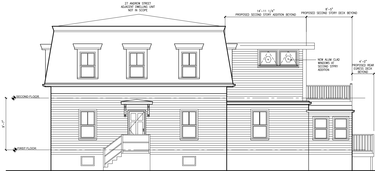
3 Existing 27 Andrew St Side Elevation (East) Scale: 1/4" = 1'-0"
