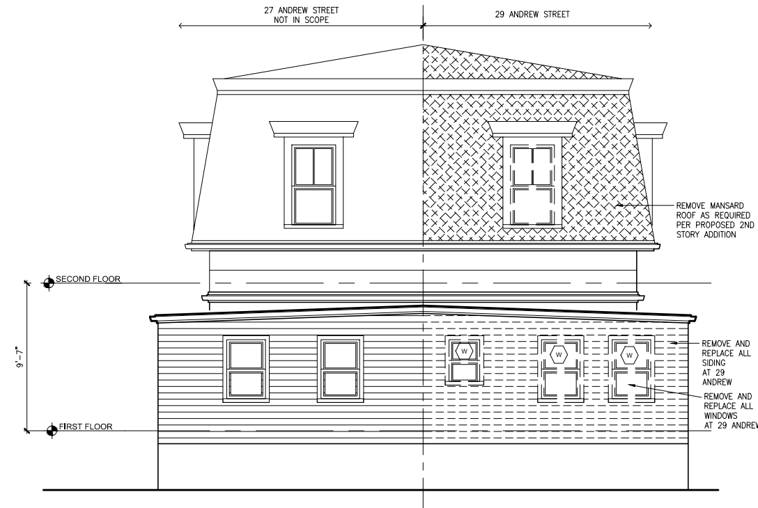
4 Existing Elevation (Rear View) Scale: 1/4" = 1'-0"
