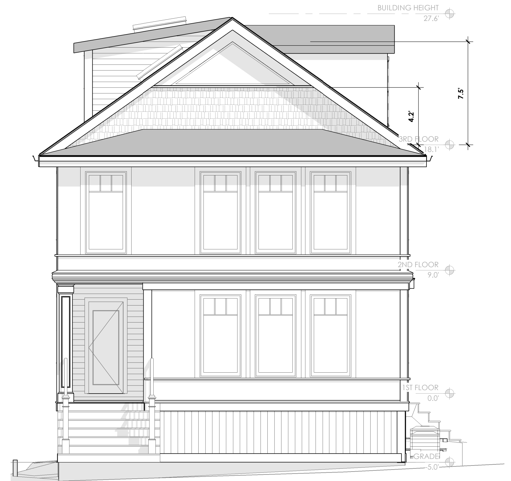
② PROPOSED FRONT ELEVATION 1/4" = 1'-0"
