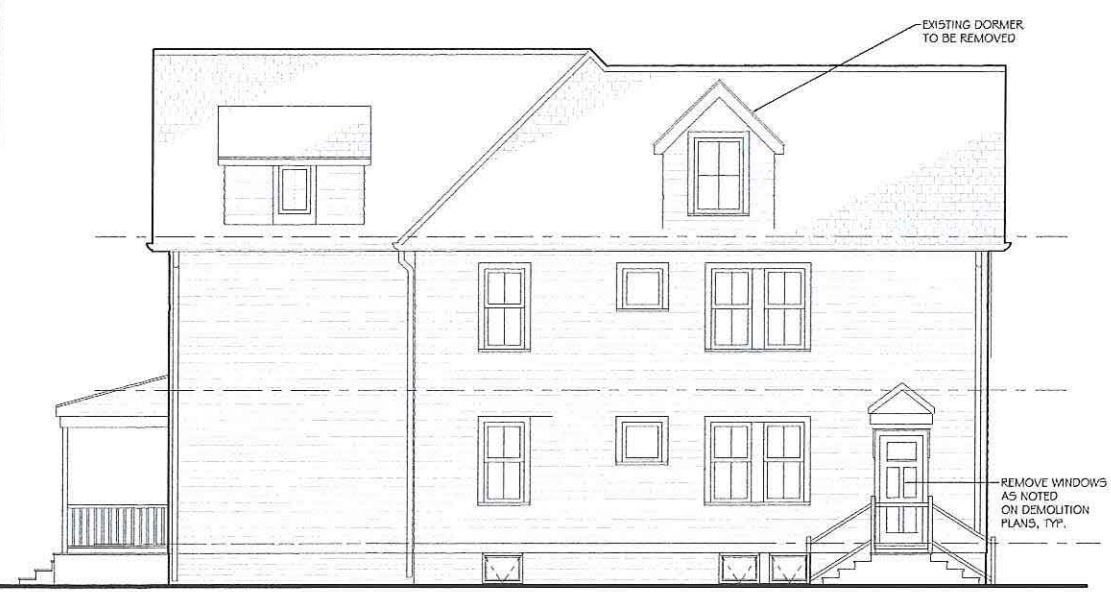
4 North Elevation - Existing Scale: 3/16" = 1'-0"
