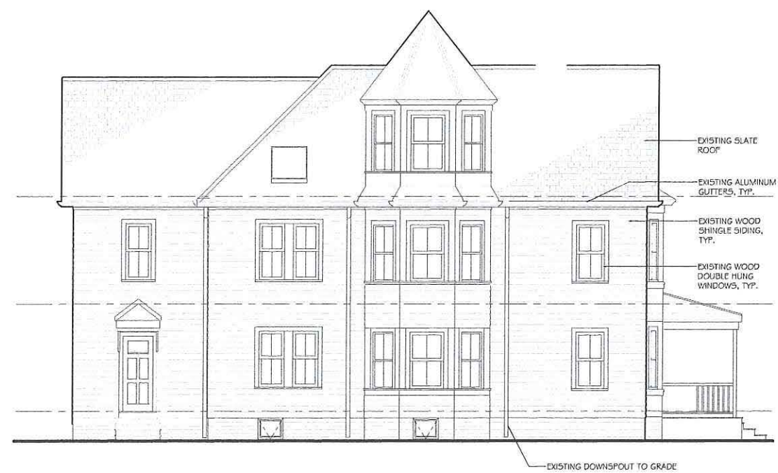
2 South Elevation - Existing Scale: 3/16" = 1'-0"
