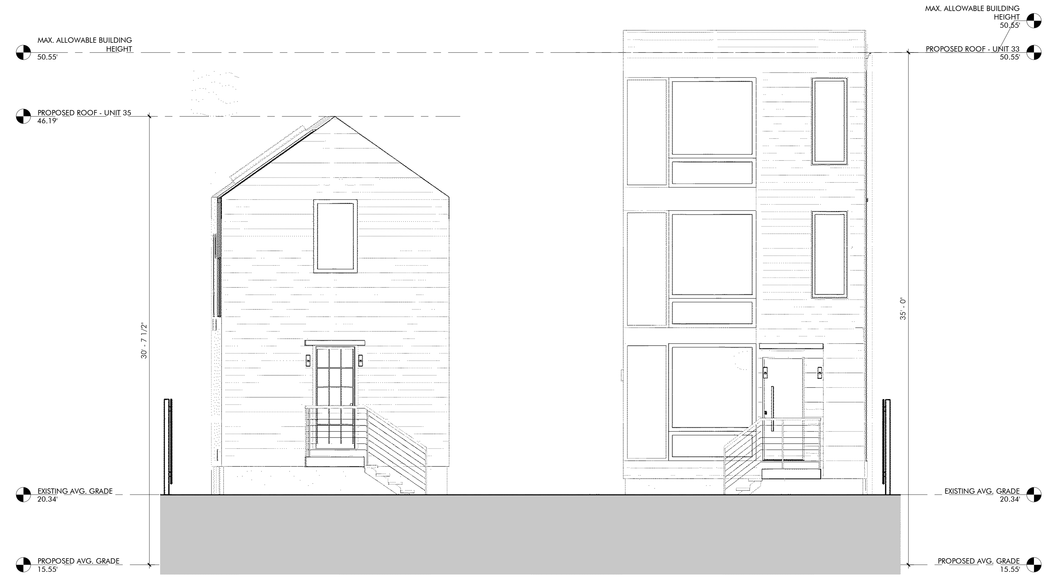
③ UNITS 33 & 35 FRONT ELEVATION 1/4" = 1'-0"
