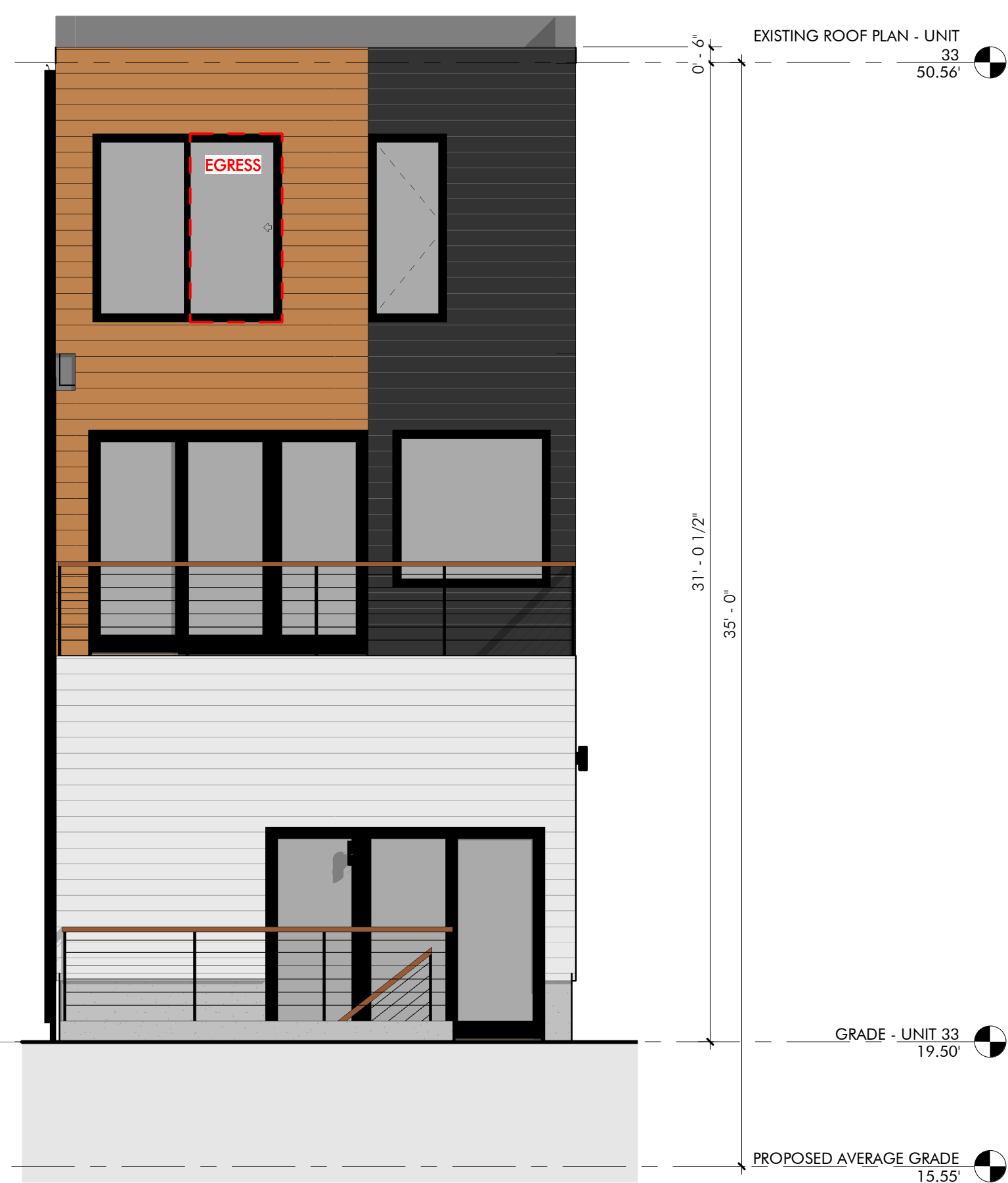
2 PROPOSED EAST ELEVATION - UNIT 33 1/4" = 1'-0"
