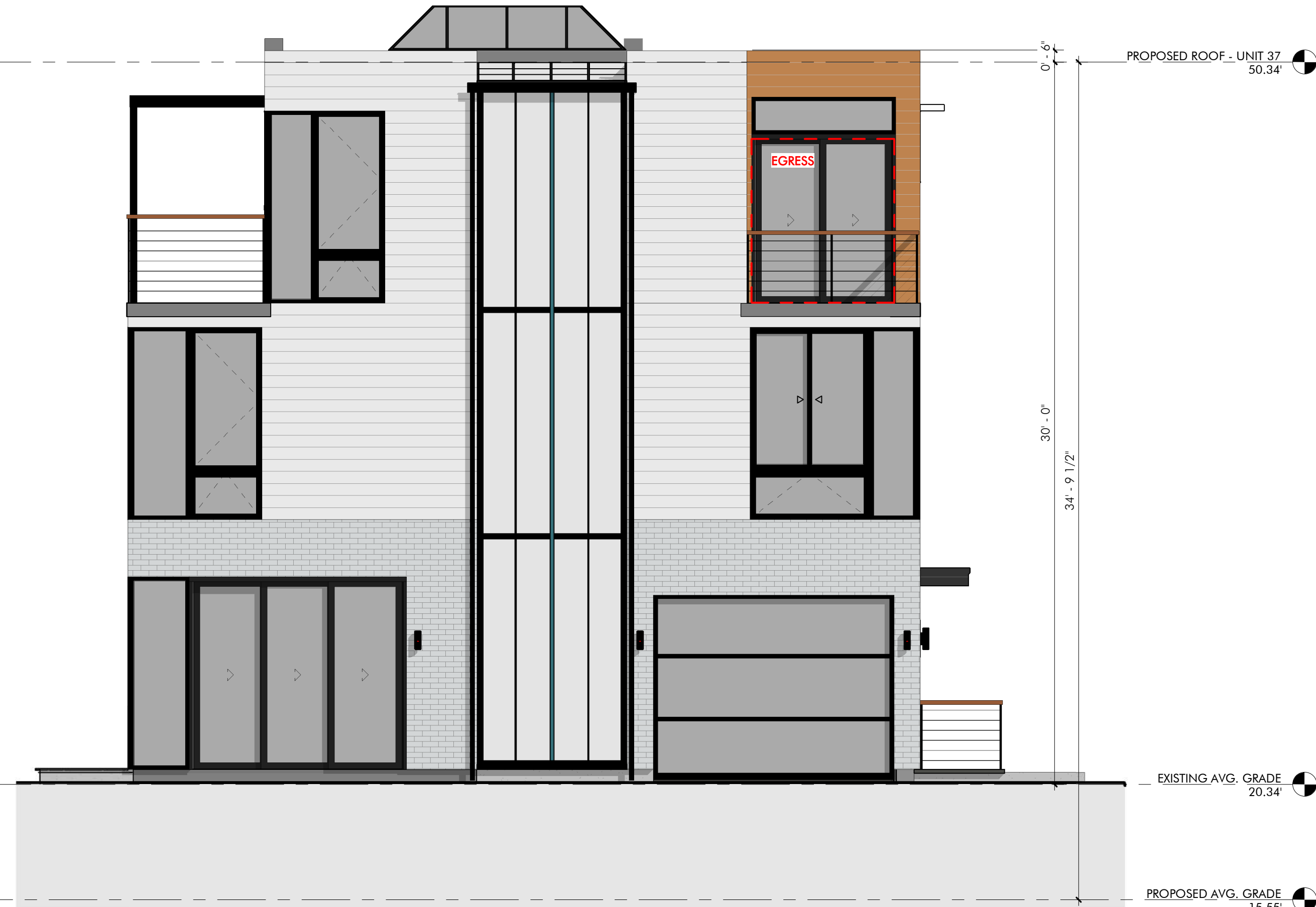
② PROPOSED EAST ELEVATION - UNIT 37 1/4" = 1'-0"
