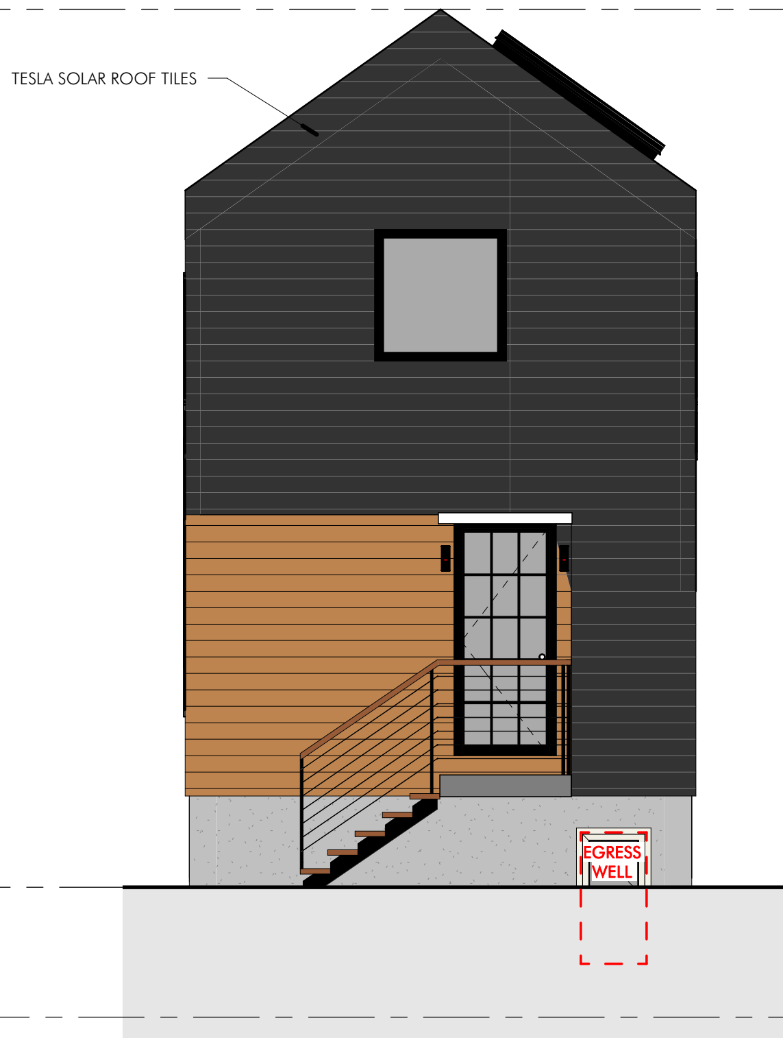
② PROPOSED EAST ELEVATION - UNIT 35 1/4" = 1'-0"
