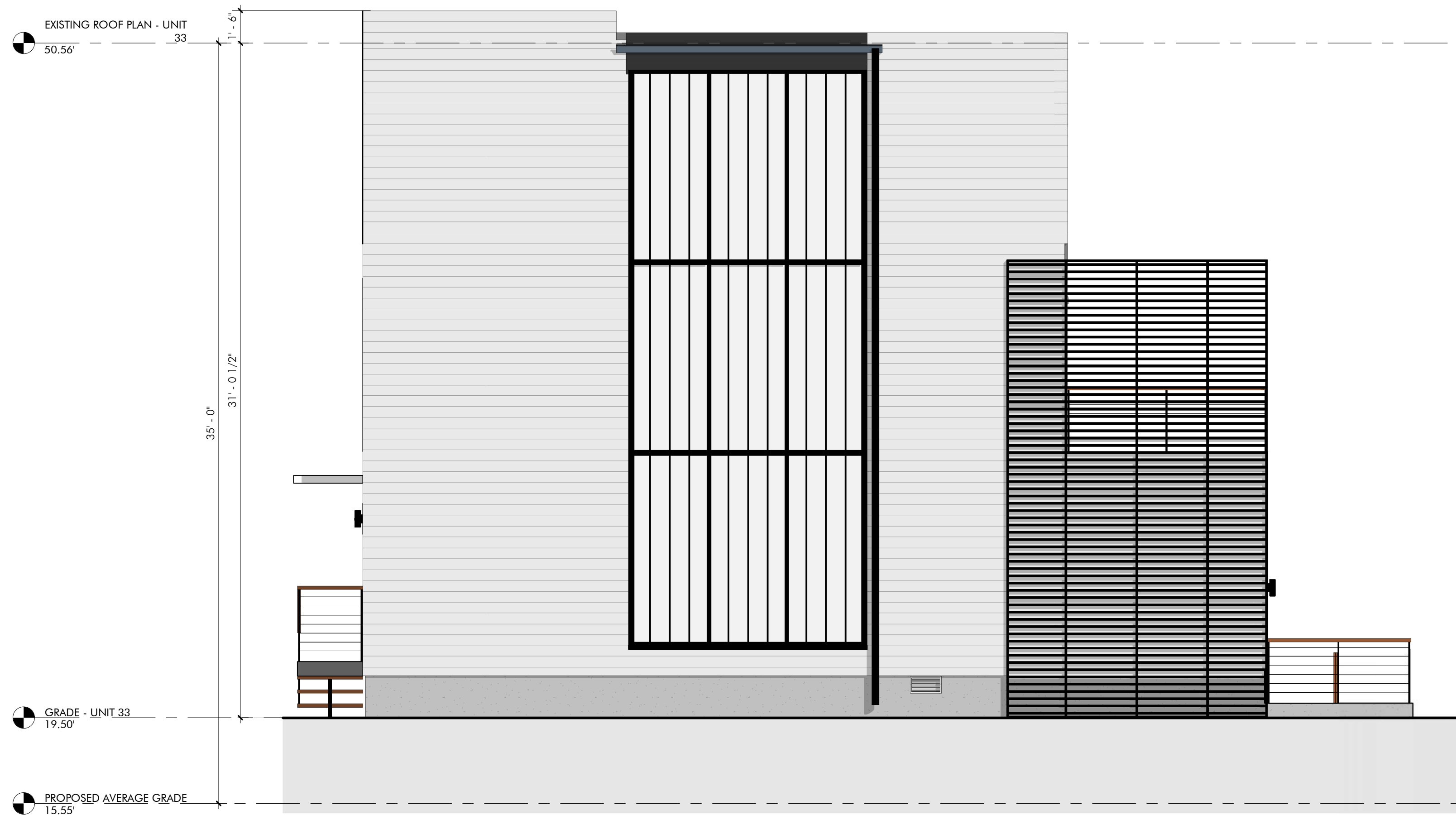
1 PROPOSED SOUTH ELEVATION - UNIT 33 1/4" = 1'-0"
