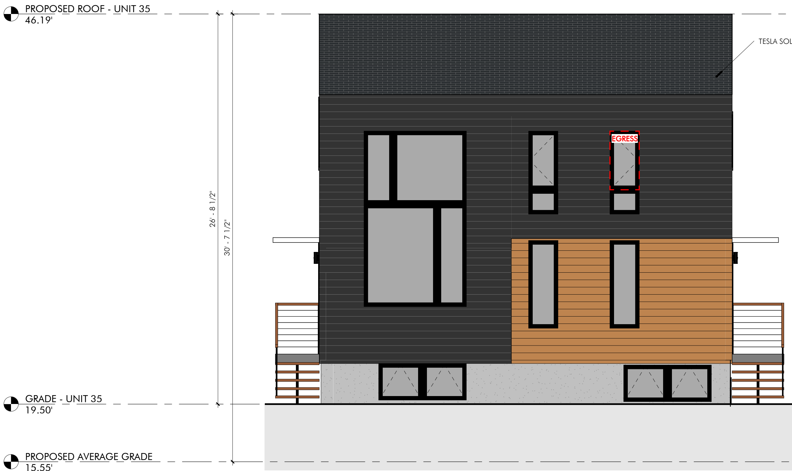
① PROPOSED SOUTH ELEVATION - UNIT 35 1/4" = 1'-0"
