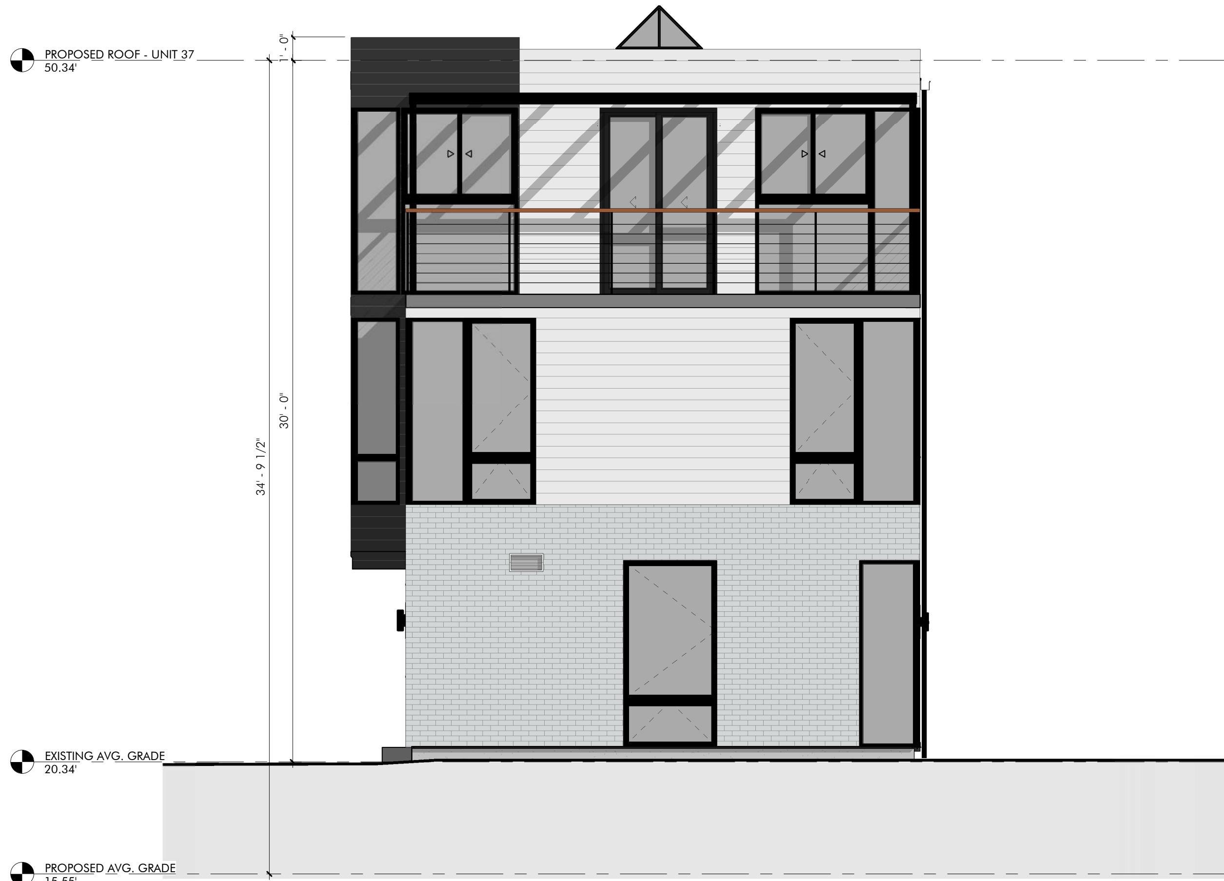
① PROPOSED SOUTH ELEVATION - UNIT 37 1/4" = 1'-0"
