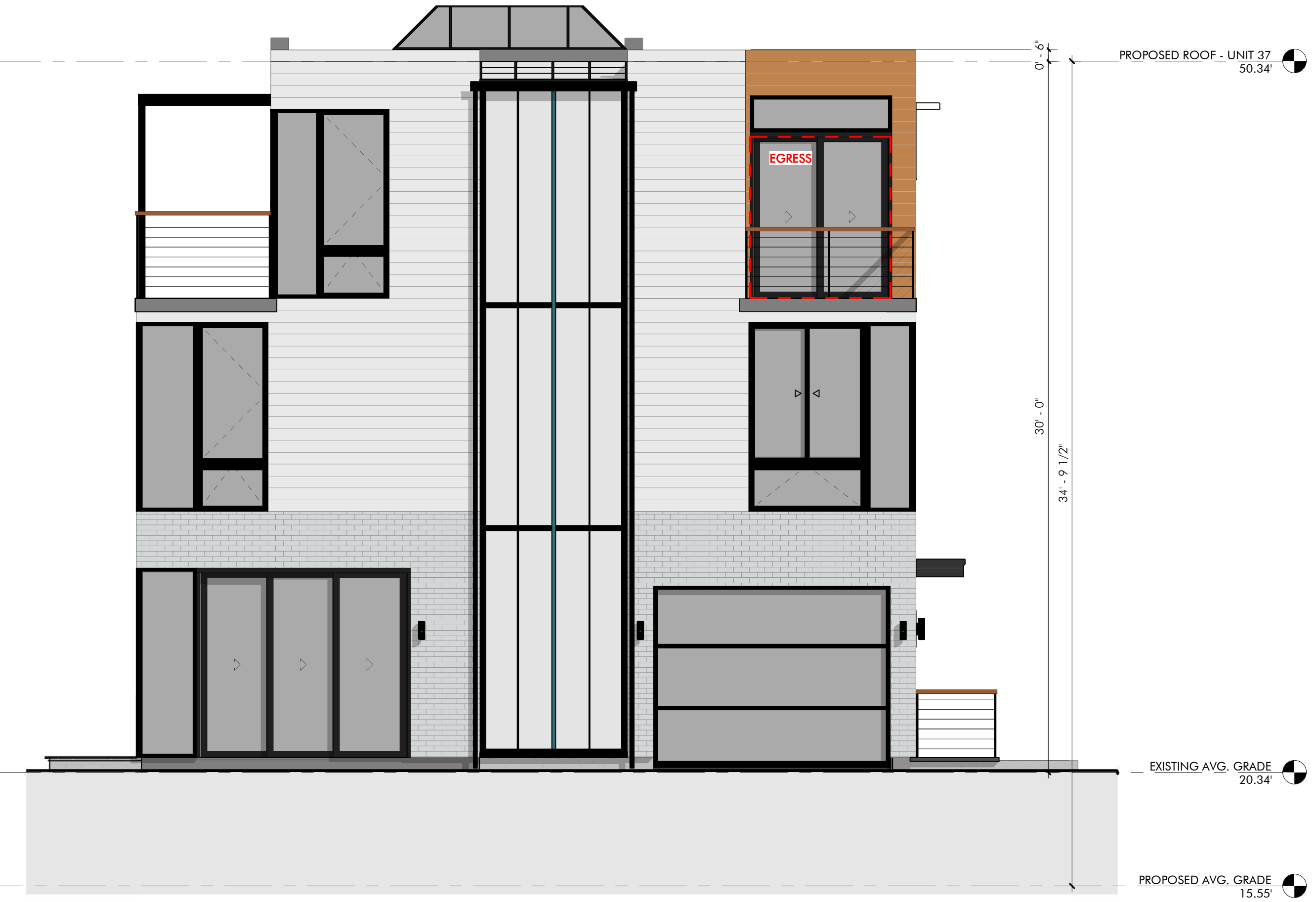
② PROPOSED EAST ELEVATION - UNIT 37 1/4" = 1'-0"
