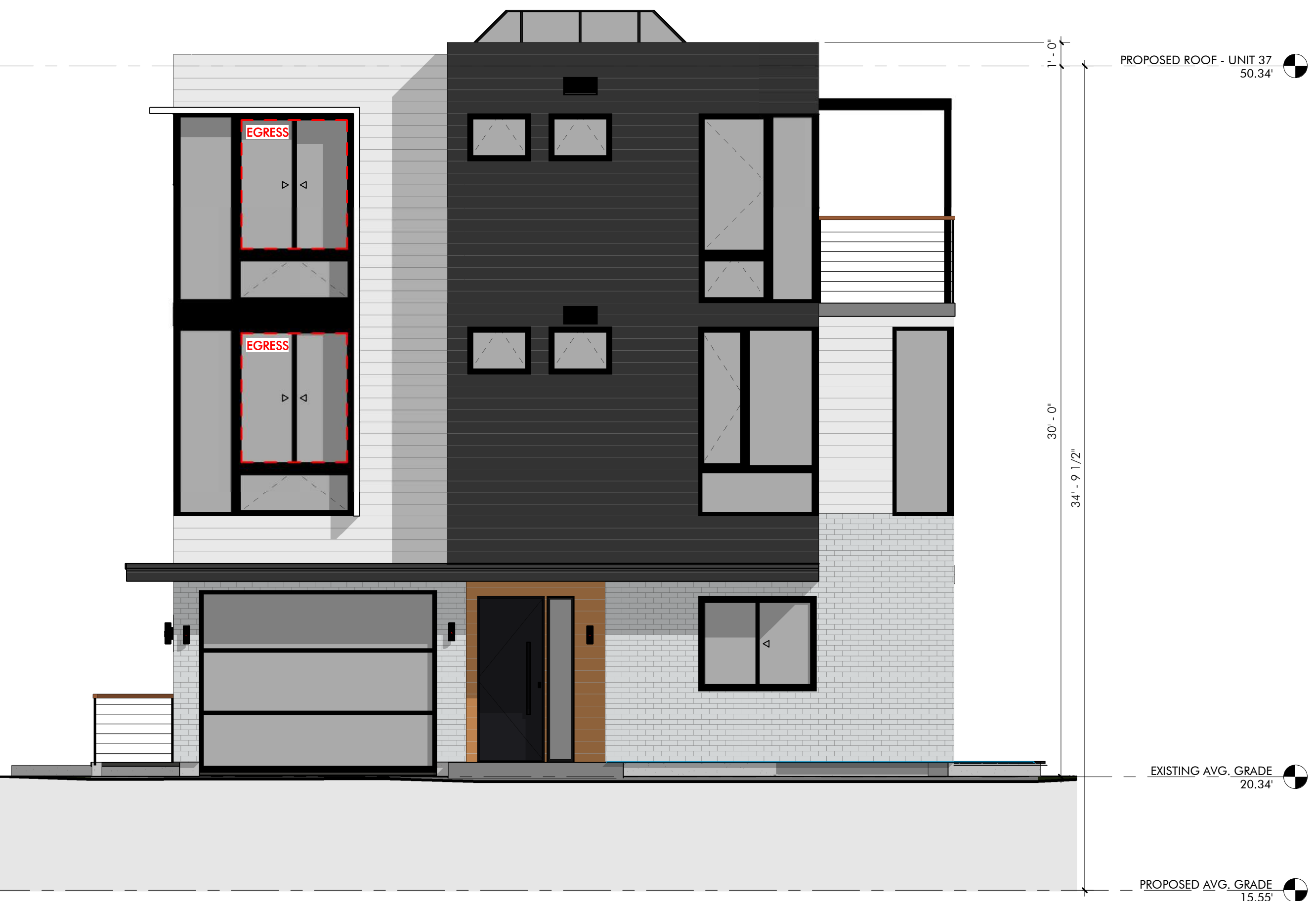
④ PROPOSED WEST ELEVATION - UNIT 37 1/4" = 1'-0"
