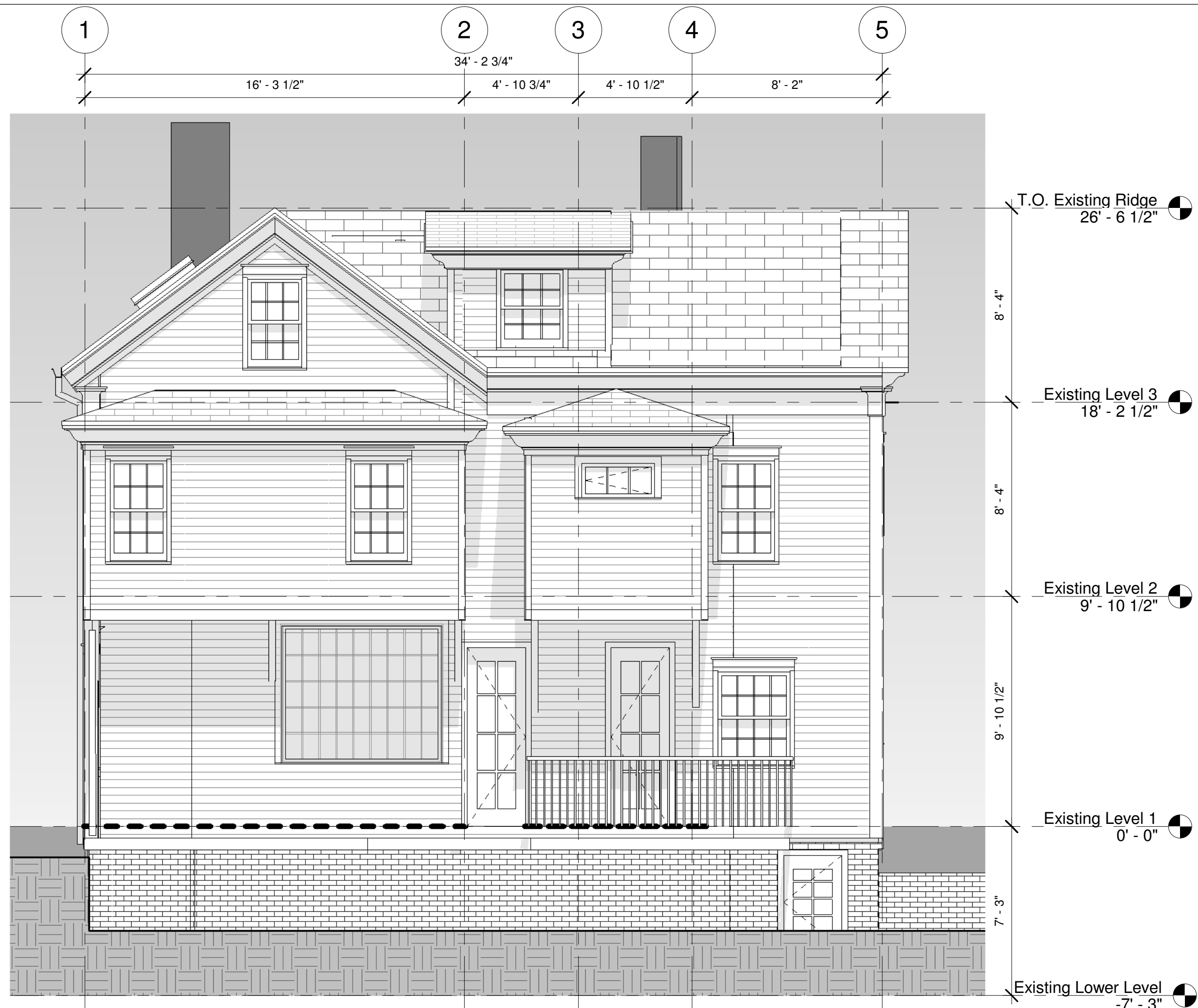
③ EXISTING WEST ELEVATION 1/4" = 1'-0"
