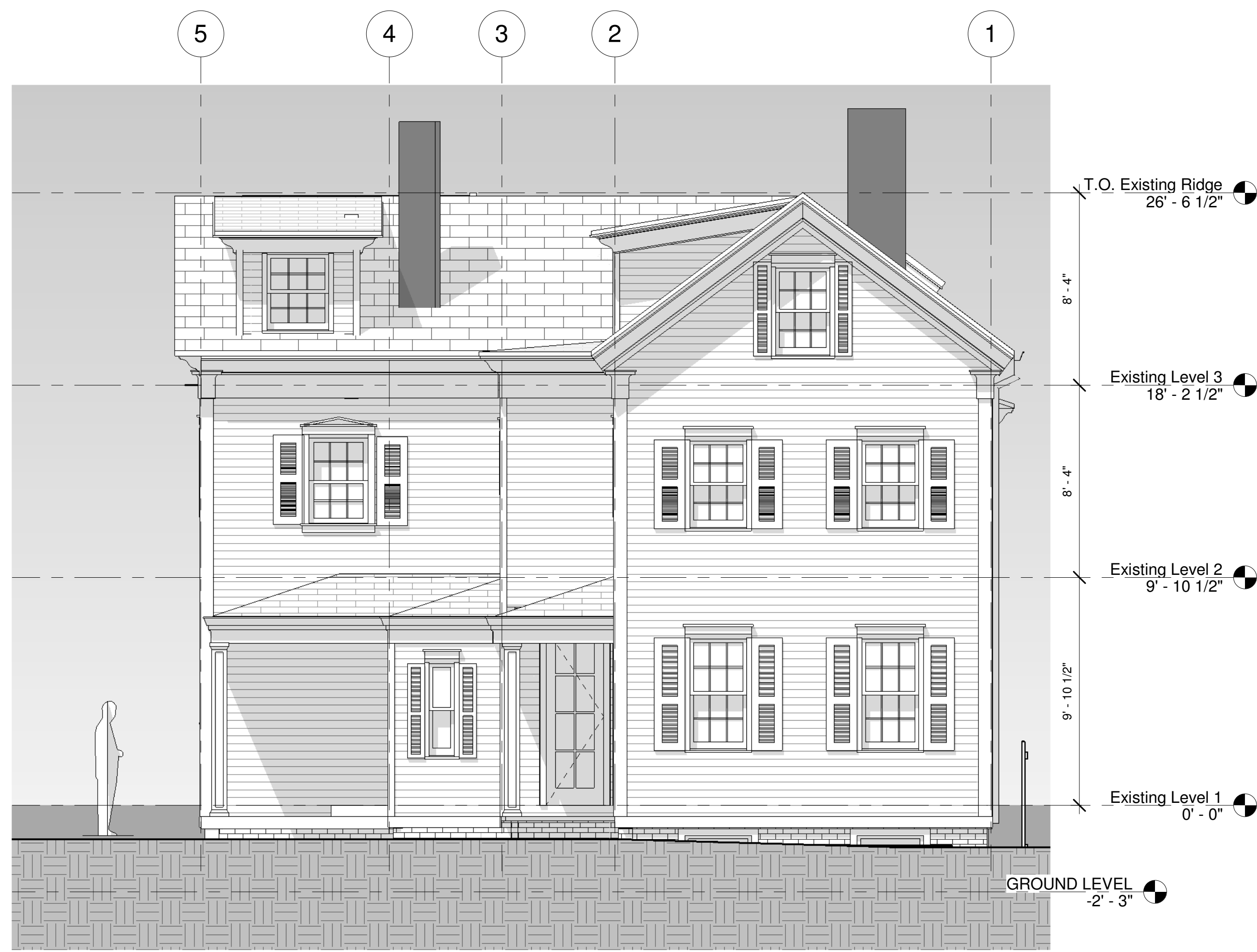
3 EXISTING EAST ELEVATION 1/4" = 1'-0"
