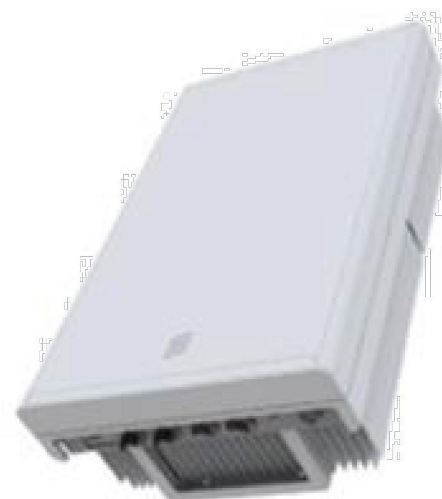
ERICSSON M-MIMO AIR6449 B77D ANTENNA DIMENSIONS: 33.1"H x 20.5"W x 8.3"D WEIGHT: 103.0 lbs QUANTITY: 1 PER SECTOR, TOTAL OF 3 SECTORS: ALPHA, BETA, GAMMA
