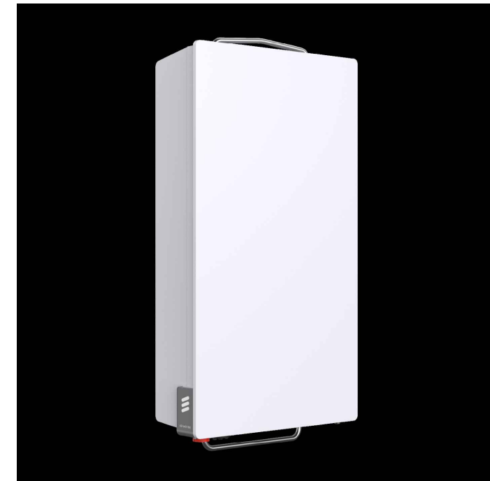
ERICSSON M-MIMO AIR6419 B41 ANTENNA DIMENSIONS: 36.3"H x 20.9"W x 9.0"D WEIGHT: 83.3 lbs QUANTITY: 1 PER SECTOR, TOTAL OF 3
