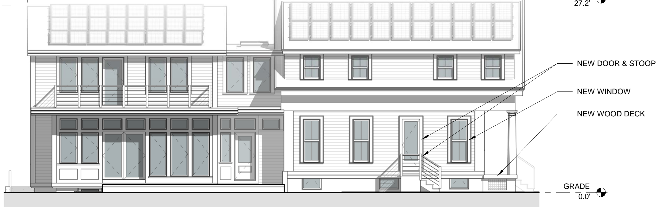
2 PROPOSED EAST ELEVATION 1/8" = 1'-0"
