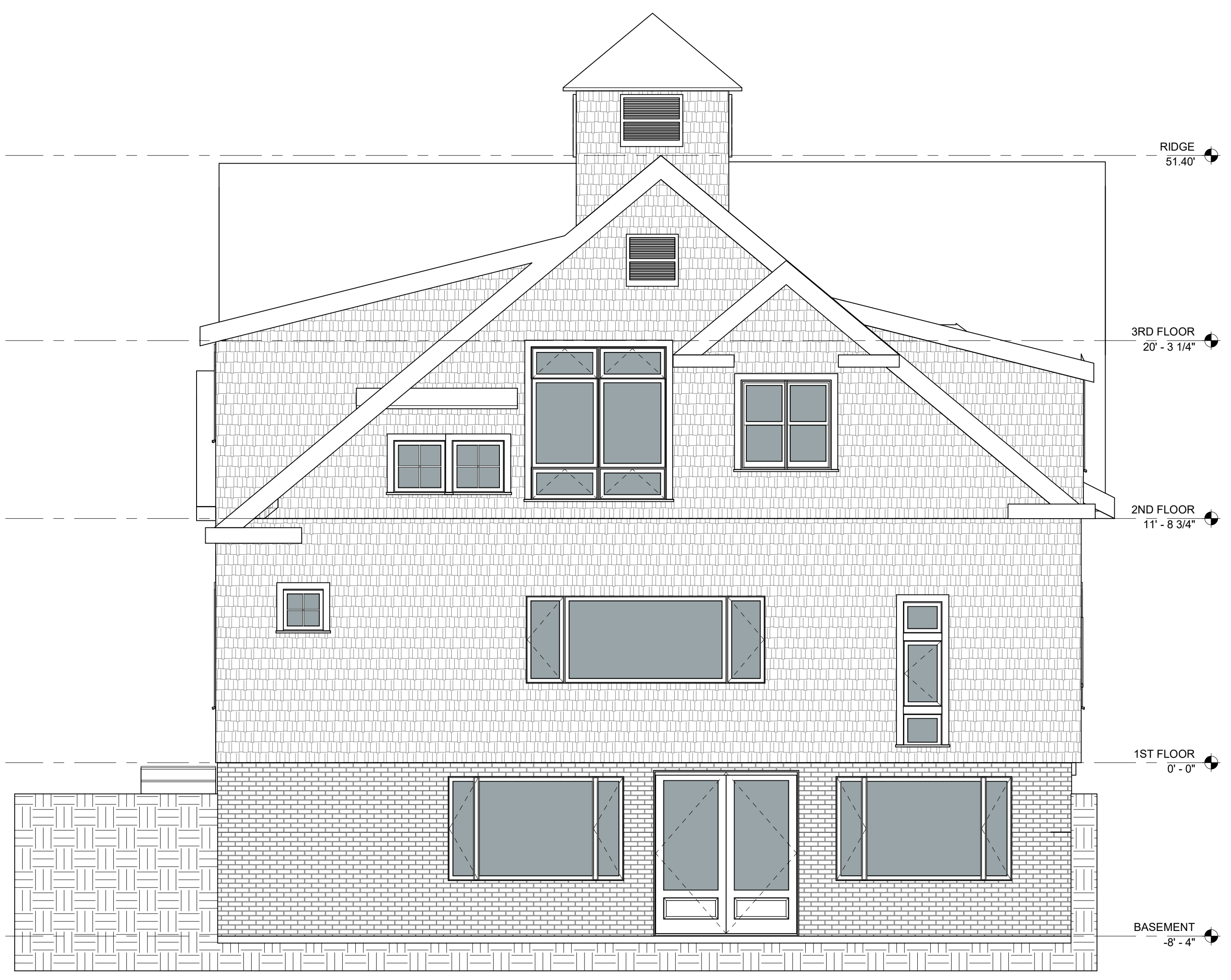
① EXISTING ELEVATION - NORTH 1/4" = 1'-0"
