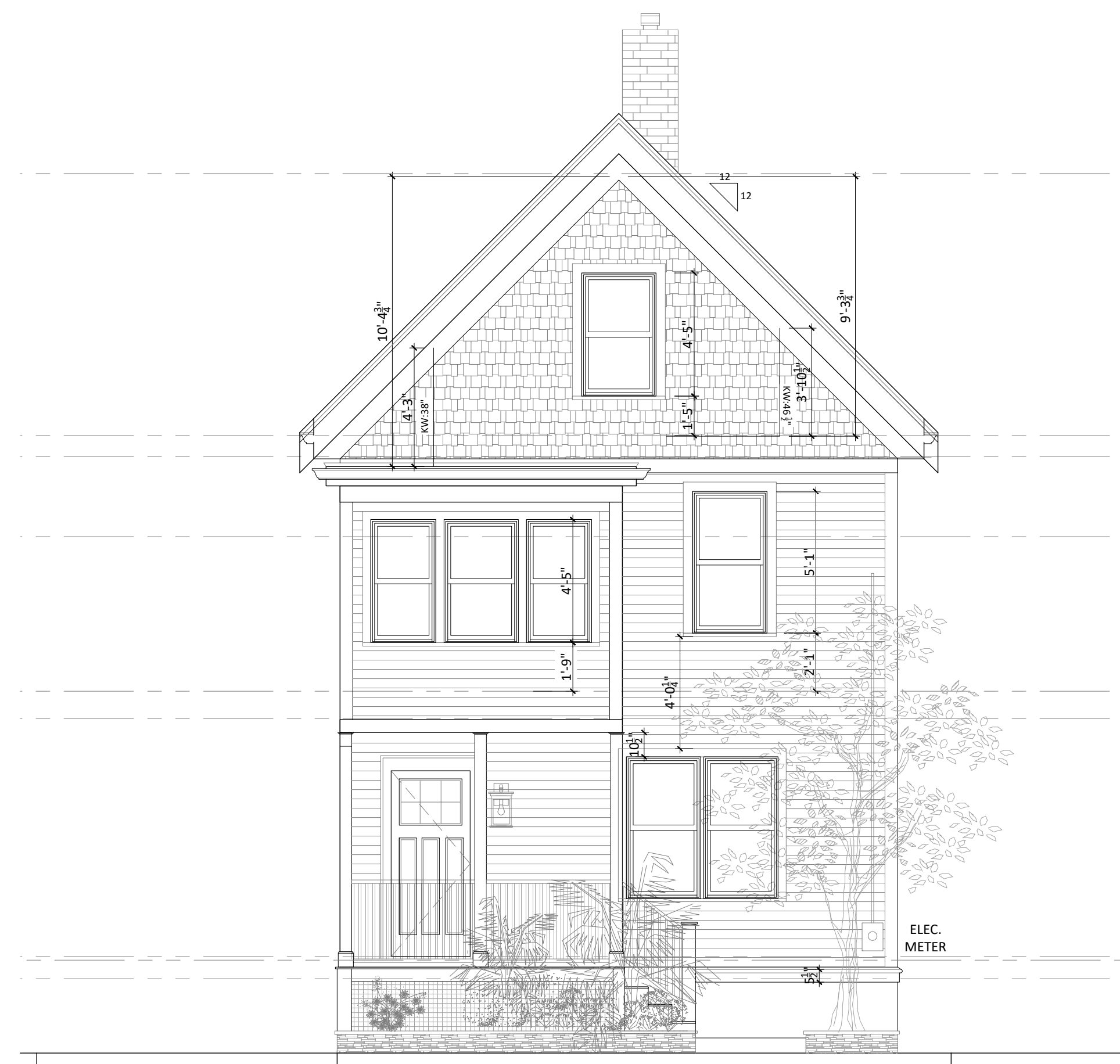
1 EXISTING CONDITIONS - FRONT ELEVATION 1/4"=1'-0"
