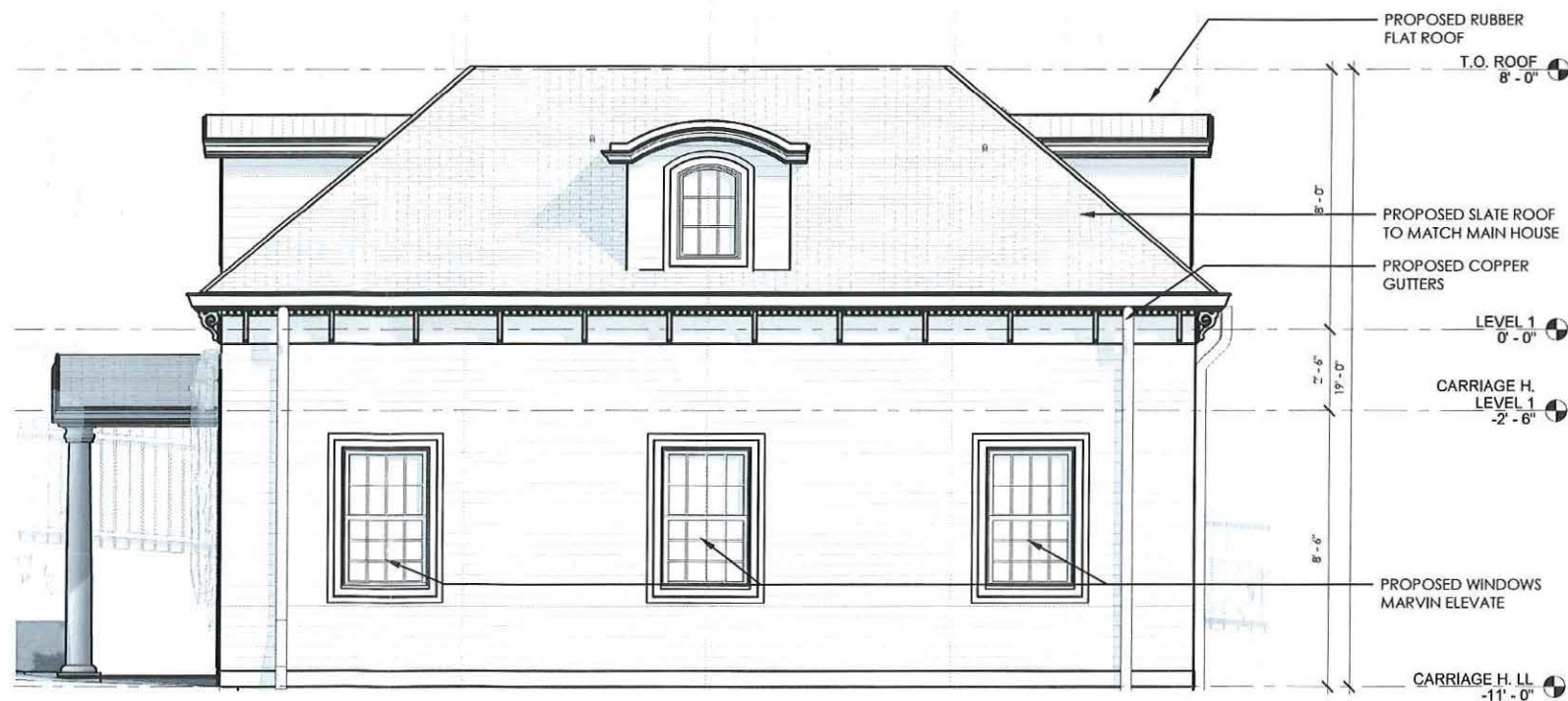
1 BZA - PROPOSED CARRIAGE HOUSE NORTH ELEVATION 3/8" = 1'-0"
